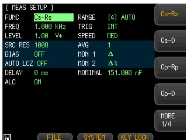
In the [MEAS SETUP] Page, you can configure each of the following measurement controls with the cursor placed in the corresponding field.
