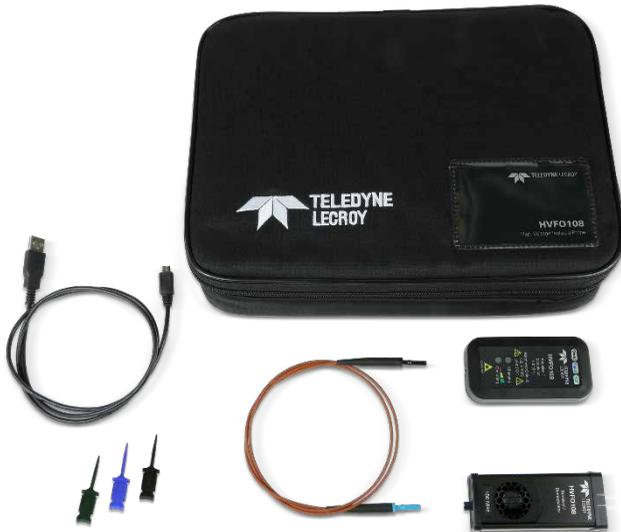
The **amplifier/modulating transmitter** is a frequency modulating optical transmitter integrated with a high-performance electrical amplifier. The transmitter is battery-powered, so there is no direct connection from the floating DUT, providing HV isolation between the device under test (DUT) and the grounded oscilloscope. The battery is recharged through the same USB Micro-B interface used to connect the tip.
