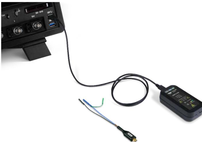
*Amplifier recharging from oscilloscope USB port.*
