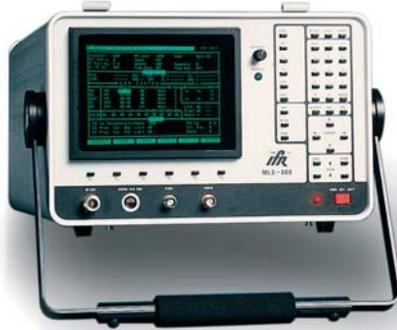
The MLS-800 provides diagnostic test capabilities for microwave landing system angle receivers.
