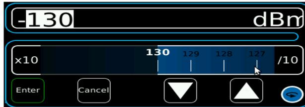
Fig. 2-9 Data Slew Bar
