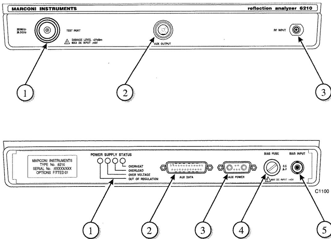
Fig. 3-9 6210 Front and Rear Panels
