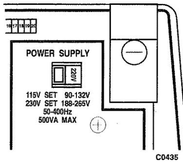
Fig. 2-1 Location of Supply Voltage Selector Switch
