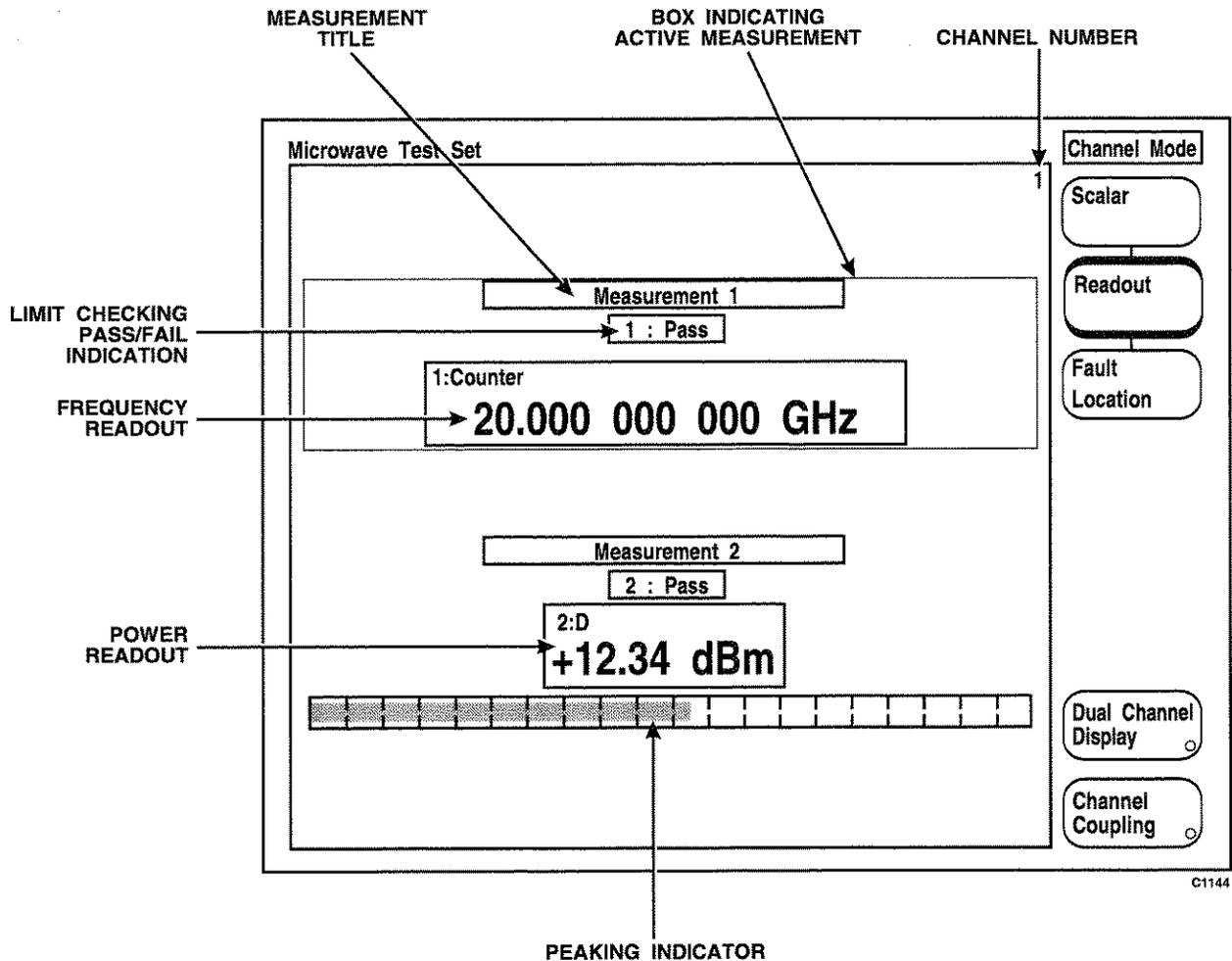
Fig. 3-5 Display - Readout Measurements
