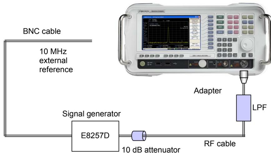
Fig. 6-16 Preamplifier test
