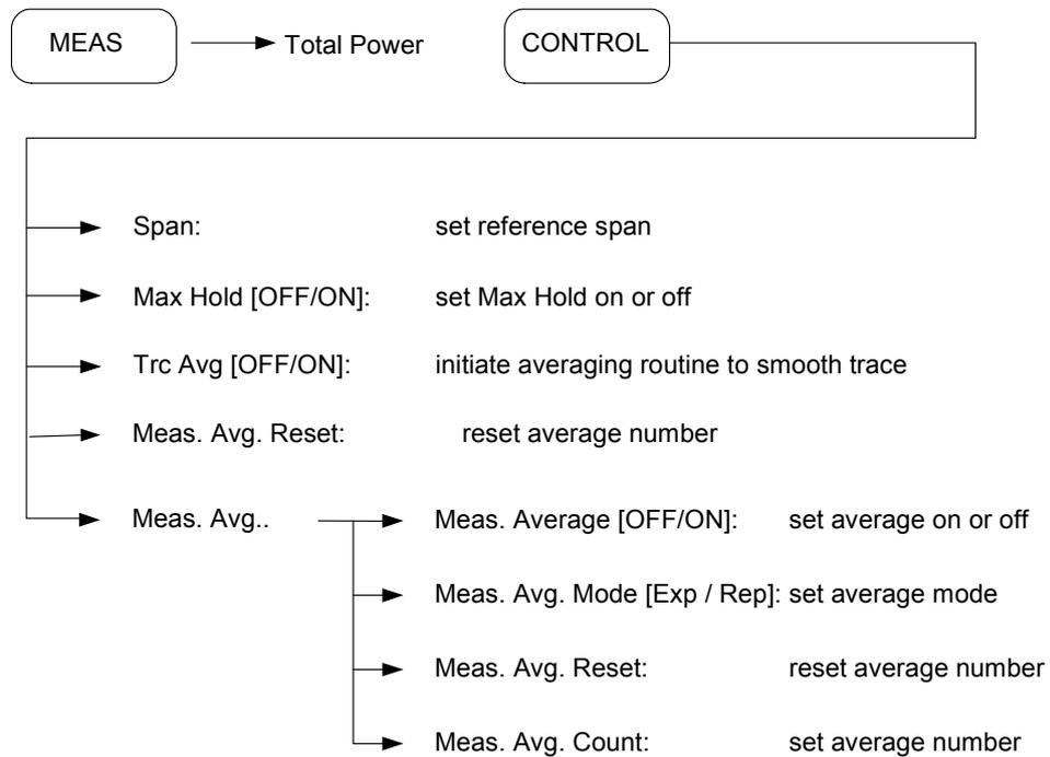
Choose the measurement configuration by using the data entry section (numeric keys, step keys or scroll knob) after each soft key [*Span*] is pressed. Adjust the BW and spacing by noting the warning or error message at the bottom of the results window.
