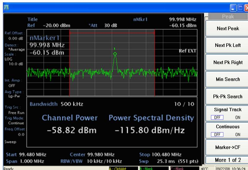
Fig. A-21 Measuring channel power
