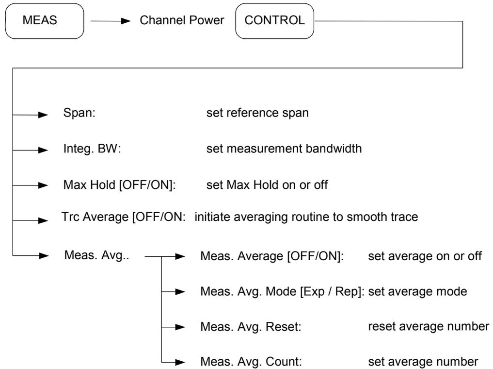
Configure the measurement by using the data entry section (numeric keys, step keys or scroll knob) after each soft key is pressed. The BW and spacing can be adjusted by observing the message at the bottom of the result window.
