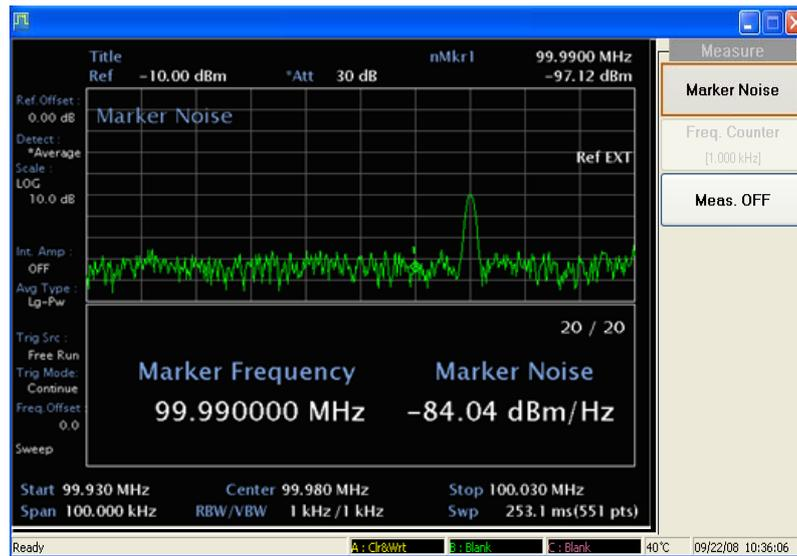
Fig. A-20 Activating the noise marker function
