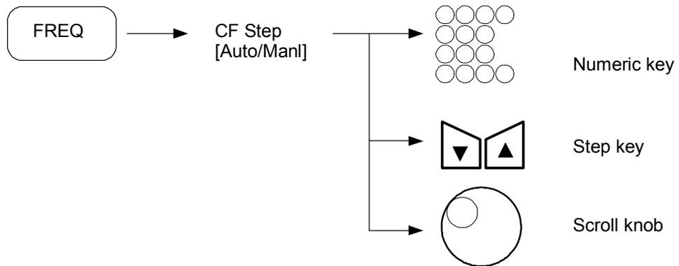
Change the CF Step mode from AUTO to MANL mode by pressing [*CF Step*].
