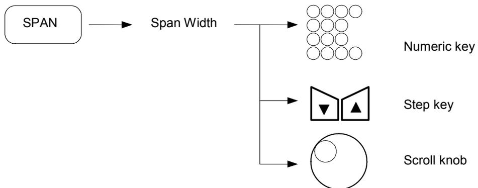
Span range is 10 Hz–3 GHz/6.2 GHz/13.2 GHz/26.5 GHz. It changes in a 1, 2, 5-step sequence: 1 k, 2 k, 5 k, ....., 100 k, 200 k, 500 k, ...
