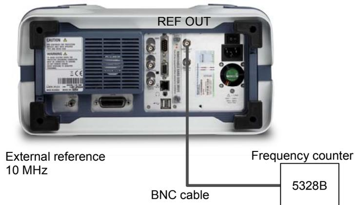
Fig. 6-2 Reference oscillator frequency stability test
