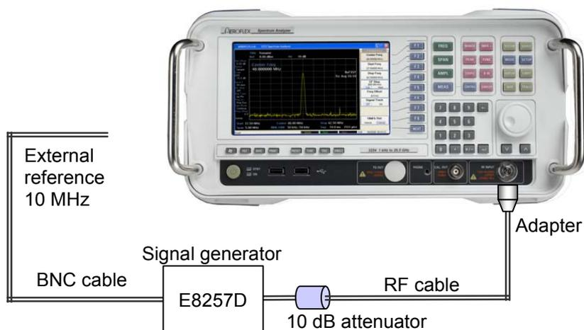
Fig. 6-5 Phase noise test
