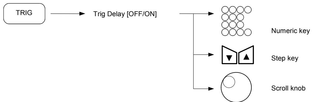
Set the delay time using numeric keys, the scroll knob and the step up/down keys in Zero Span mode. The range of delay time is (-150 ms to +500 ms).
