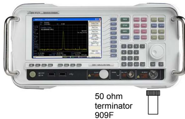
Fig. 6-7 Average noise level test
