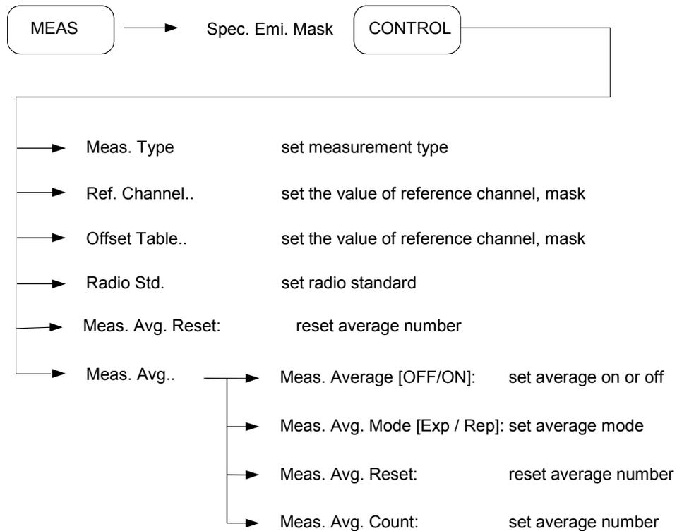
The measurement type is either Total Pwr Ref method using Total Power or PSD Ref method using Power Spectral Density.
