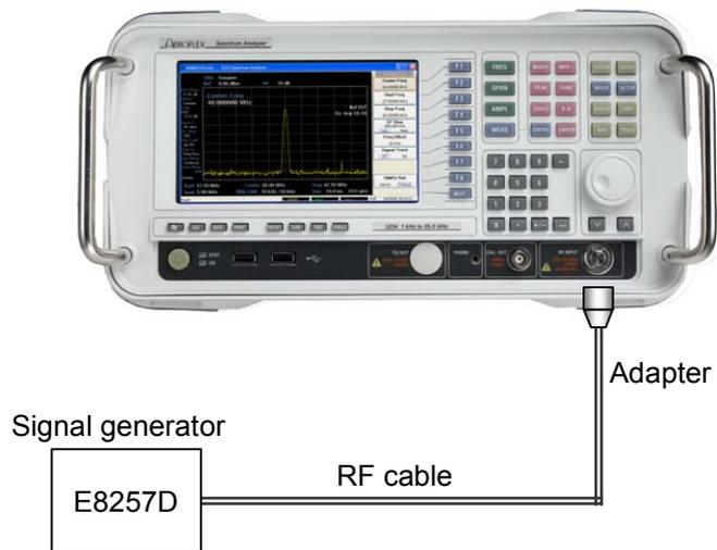
Fig. 6-6 Residual FM test
