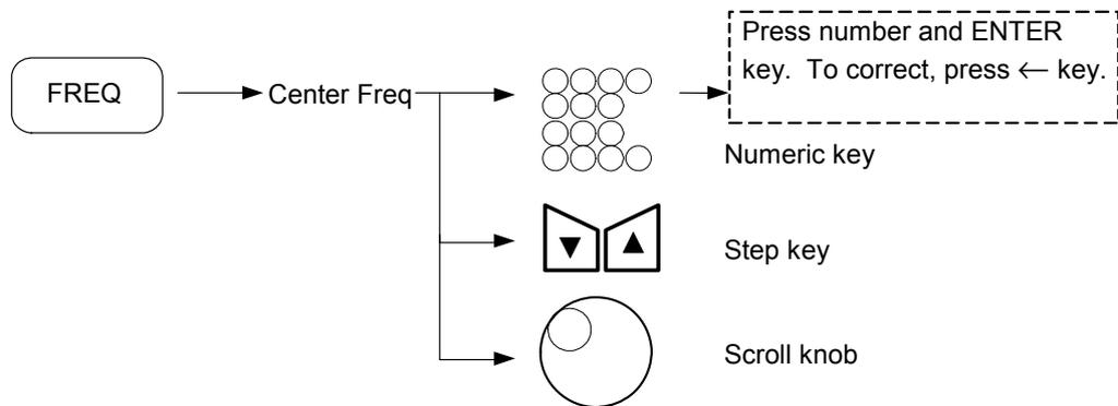
The step size of the step up/down key is 1/10 of the current frequency span (CF Step mode set to [MANL](#), page 5-11).
