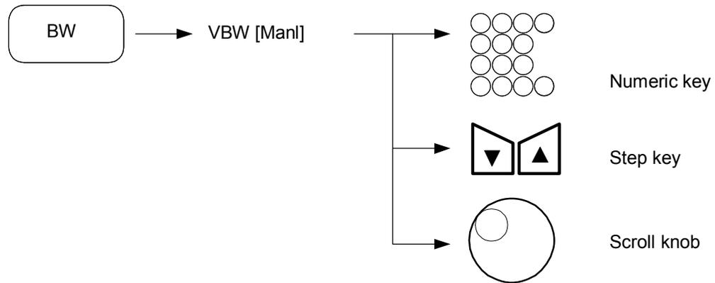
Use the MANUAL setting to average noise by making the VBW narrow without regard to the RBW value, or when wanting to make the VBW wide to observe the waveform of signals modulated at a high frequency. The VBW value can be manually set from 1 Hz to 3 MHz in 1, 2, 3, 5 steps.
