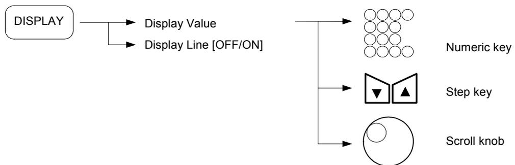
The step size of the step up/down key is one division of the vertical range.
