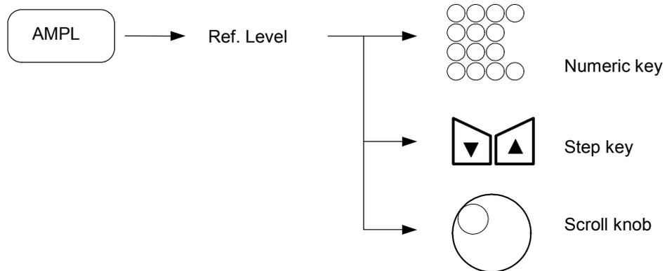
The step size is one division of the current scale (see [Setting Amplitude Scale](#) on page 5-15).
