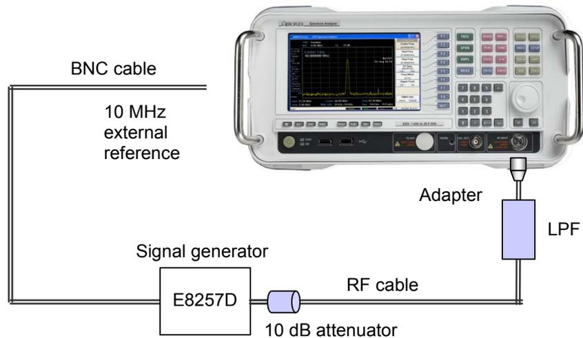
Fig. 6-13 Spurious relating to input test
