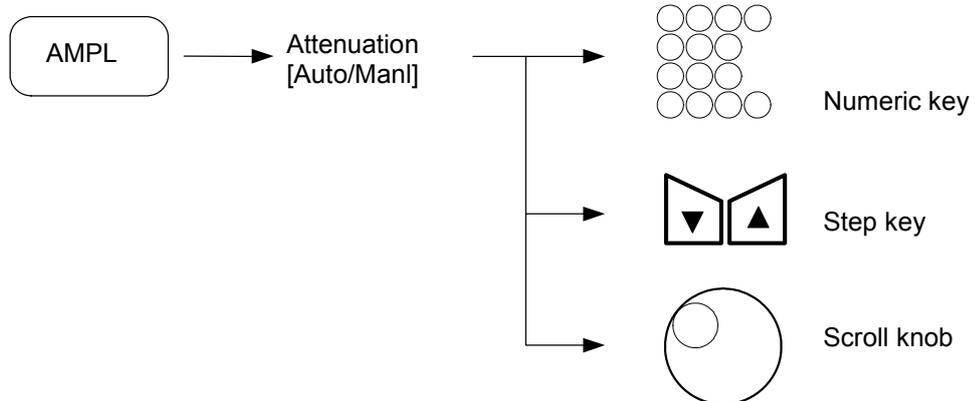
Change the Atten. mode [AUTO or MANL] by pressing [*Attenuation [Auto/Manl]*]. In Atten MANL (manual) mode, the step size of the input attenuator can be set by the numeric keys, step keys, and scroll knob (range 0 to 55 dB) (see [Input Attenuator](#) on page 5-19).
