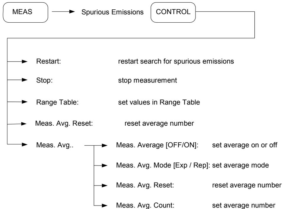
Using the range table, you can distinguish a total of 200 ranges (range setting duplicates allowed) and set ranges such as RBW, VBW, sweep time, input attenuation and peak parameters.
