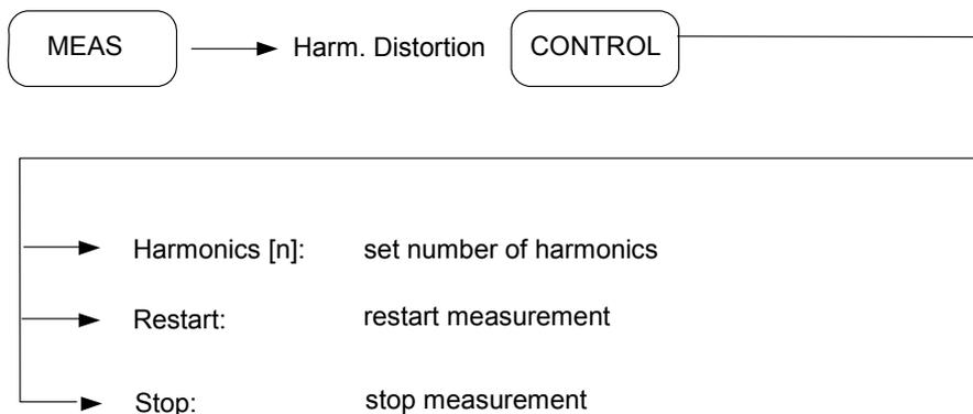
‘Harmonics number’ means the number of nth harmonics. The harmonics number can be set between 2 and 5; the default is 5. The recommended SPAN value is less than 4 MHz for an accurate measurement.
