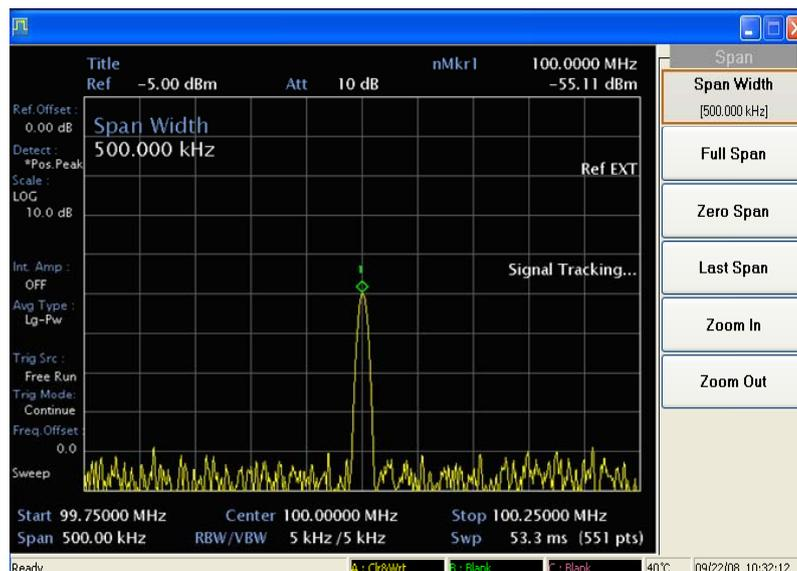
Fig. A-7 Using marker counter
