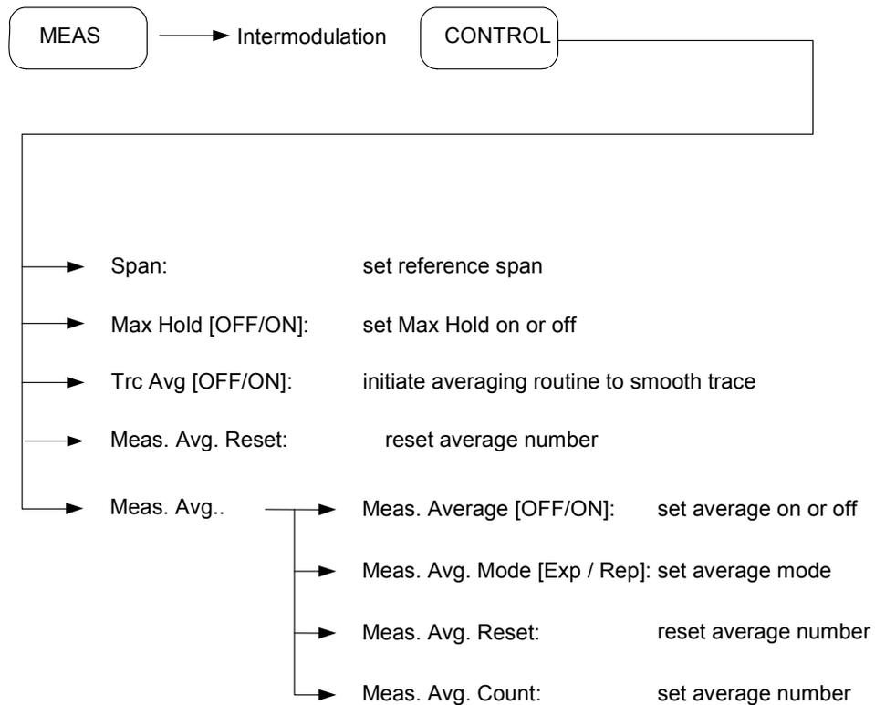
Choose the measurement configuration by using the data entry section (numeric keys, step keys or scroll knob) after each soft key [*Span*] is pressed. Adjust the BW and spacing by noting the warning or error message at the bottom of the results window.
