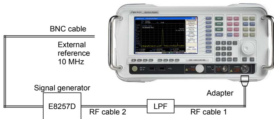
Fig. 6-11 Second harmonic distortion test
