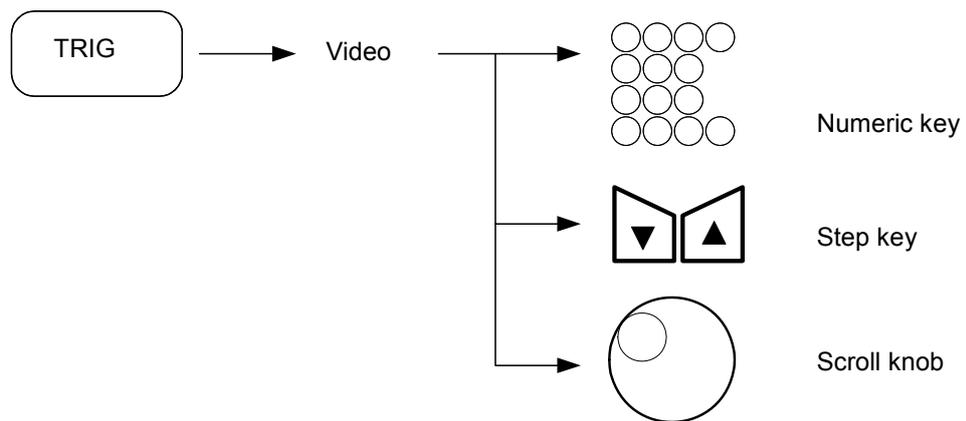
The trigger level is controlled by the step up/down keys or the scroll knob.
