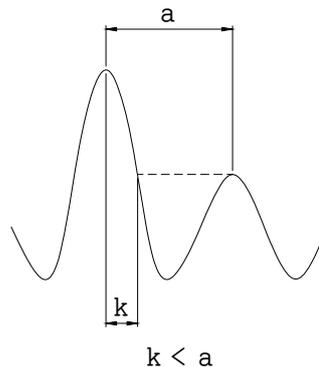
Fig. A-4 Resolution bandwidth requirements for resolving small signals
