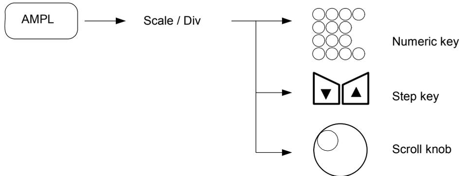
The amplitude scale is changed into a 1, 2, 5 step sequence by pressing the step key.
