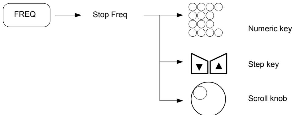
The step size of the step up/down key is 1/10 of the current frequency span.
