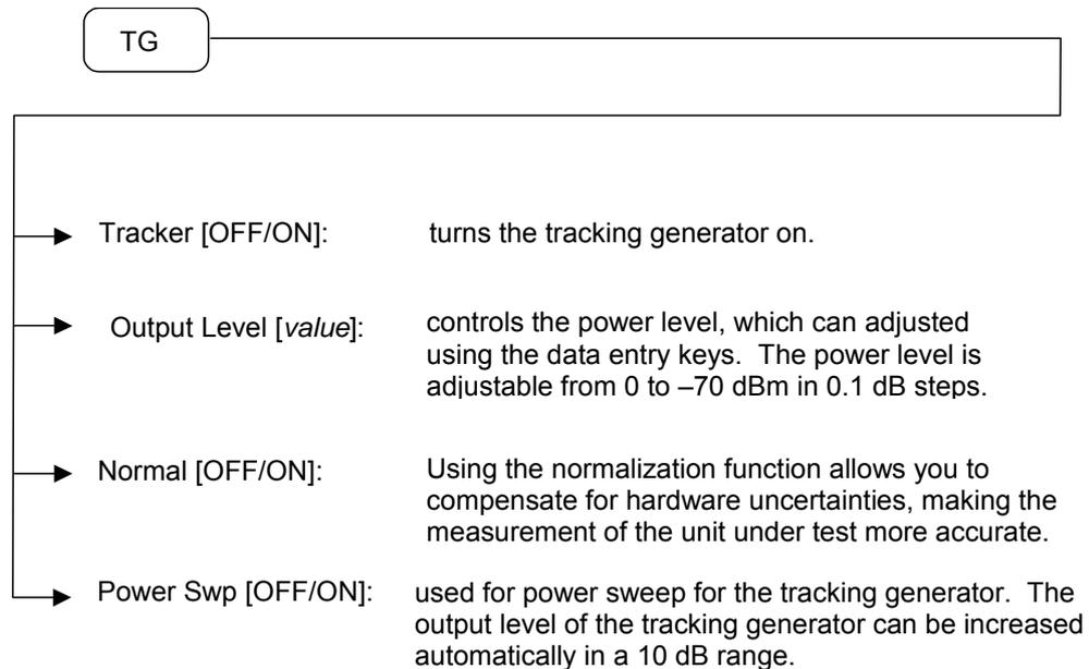
The *Normal* menu provides for a more convenient measurement by normalizing the unloaded output signal.
