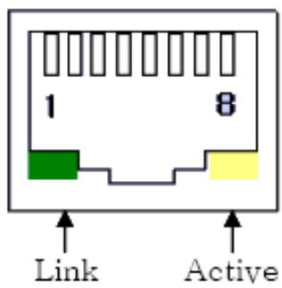
Fig. 3-7 ETHERNET connector
