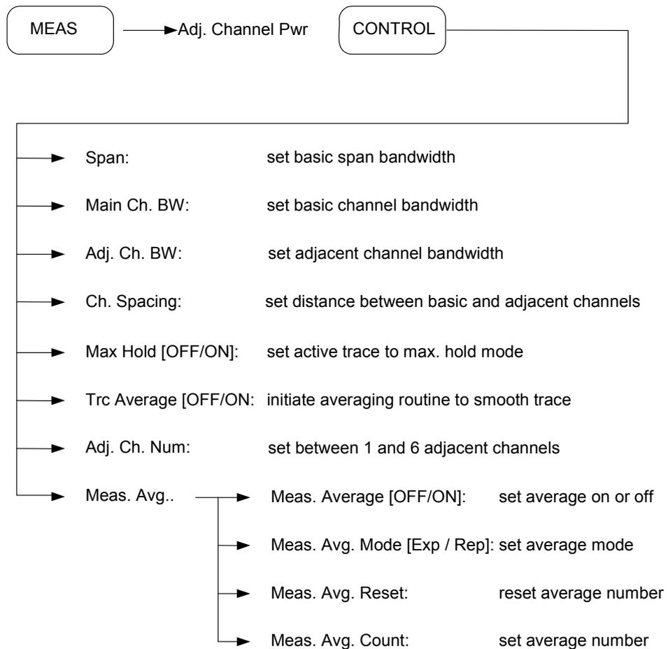
Measurement configuration is done by using the data entry section (numeric keys, step keys or scroll knob) after each soft key [*Main Ch. BW*], [*Adj. Ch. BW*], [*Ch. Spacing*] is pressed. Adjust the BW and spacing by observing the messages at the bottom of the result window.
