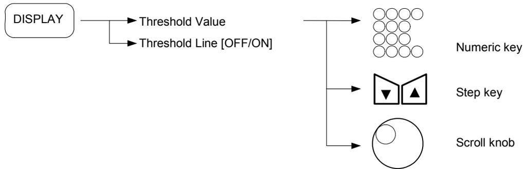
The step size of the step/up down keys is one division of the vertical range.
