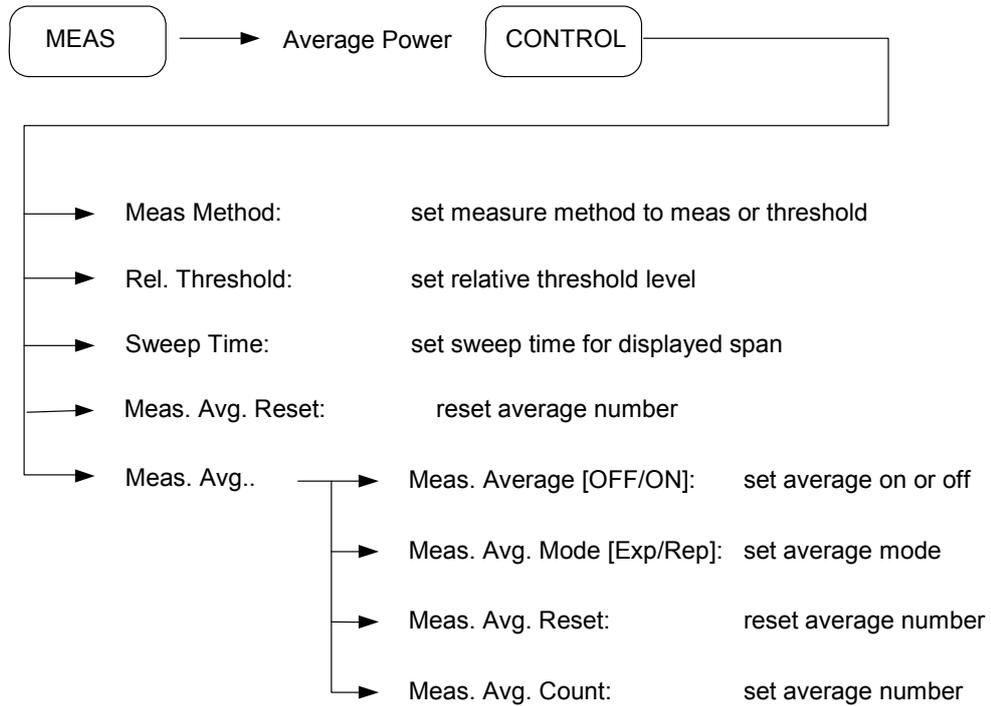
To measure Average Power, set the span to zero span at the current center frequency. You need to have set the center frequency and reference previously.
