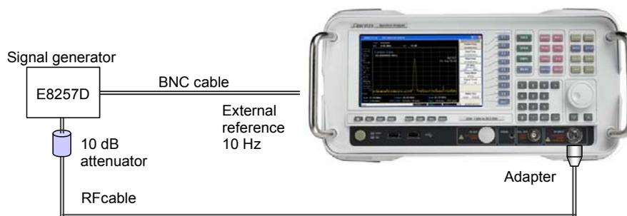
Fig. 6-8 Input attenuator switching error test
