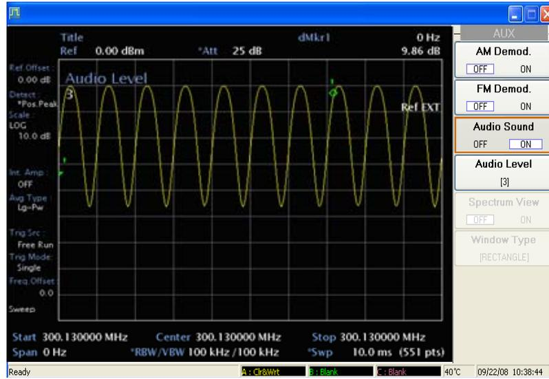
Fig. A-27 Measure the demodulation in zero span
