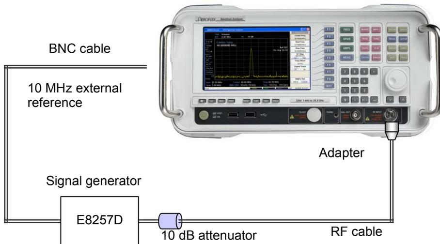
Fig. 6-3 Frequency counter accuracy test
