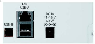
The 2201 ProLock can be operated from an external DC source such as the power supply which is delivered with ProLock, or a car battery. The DC voltage must be in the range from 11 to 15 V. The power consumption may be up to 40 W.
