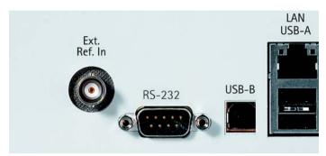
This 9-pin sub-D connector on the rear panel of the 2201 ProLock can be used to control ProLock remotely via serial interface (RS-232). The command set and the responses conform to the SCPI standard and are explained in the user's guide.
