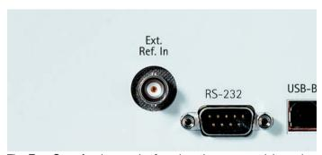
The **Ext. Sync In** plug can be found on the rear panel. It can be used as an input for an external time base (reference clock). If an external 10 MHz clock is connected, ProLock will automatically use this clock as a frequency reference, and display a symbol on the LCD screen. See the user's guide for more details.
