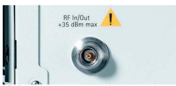
$\mbox{\bf RF in/out}$  is a 50  $\Omega$  N-type connector (female) on the left-hand side of the rear panel.
