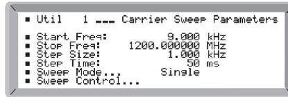
The frequency sweep facility is particularly well suited to EMI testing. During a frequency sweep, the RF level can be altered using the rotary control to manually correct the level at the output of amplifiers. The square wave modulation source allows the generation of square wave amplitude modulation to simulate the effect of TDMA bursts from communication systems on devices being tested for EMI.
