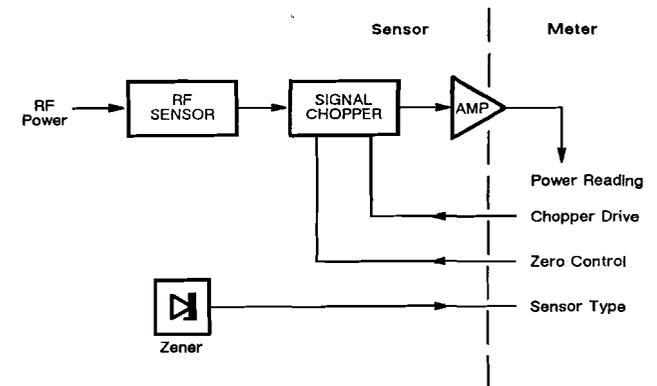
*Fig. 4-1 Block Diagram of RF Power Sensor*
