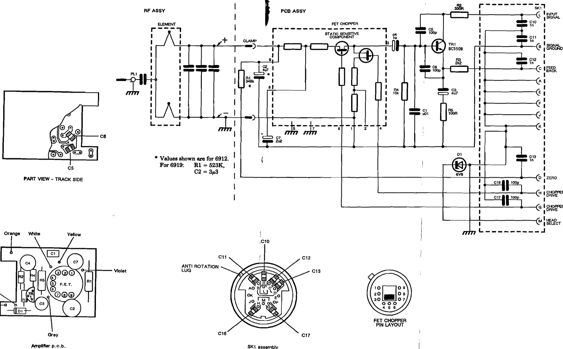
Fig. 7-3 Circuit diagram and component layout: 6912/6919
