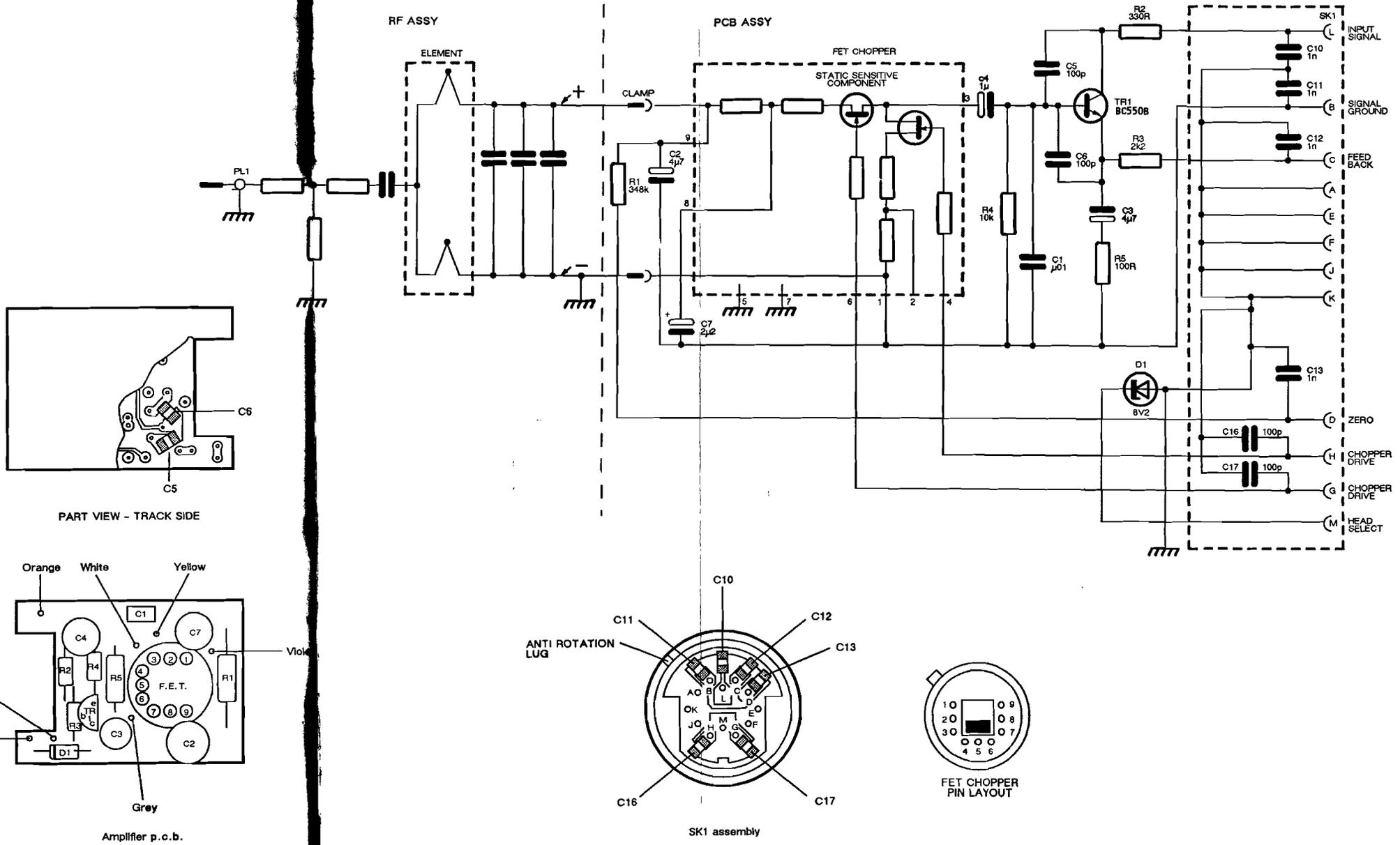
Fig. 7-6 Circuit diagram and component layout: 6932.
