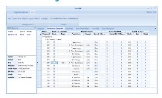
Configure Channels menu in the Scan mode can be used to enable channels as well as to configure various settings such as measurement function, range, speed of measurement. Channels can also be monitored within the defined limits by using Alarm Limit feature.
