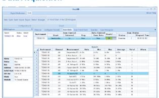
Different measurement settings such as Scan interval, Start and Stop time can be set from the Scan Data menu. The Result section provides the live measurement data along with min, max and average values. It also provides total number of scans and number of Alarm for every channel.
