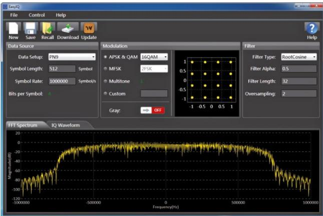
The EasyIQ software is necessary to generate an IQ waveform when using the T3AFG-IQ option.
