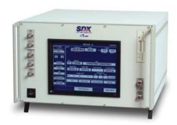
ATC, DME, Mode S, Data Link, IFF and TACAN capability in a single tester
