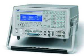
Desktop and rackmountable digital testers for PCM and data applications up to 34 Mbit/s including mux/demux
