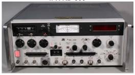
The <u>IFR RD-300</u> is designed as a precision simulator-tester of aircraft weather radar instruments. The RD-300, in conjunction with the oscilloscope, can perform virtually all routine radar testing. Because the RD-300 is connected to the unit under-test through just one calibrated coaxial cable, there is no need to reconfigure the test equipment to measure different parameters.
