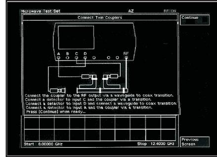
Connection diagram for measurement of return loss and insertion loss in a waveguide feed using couplers
