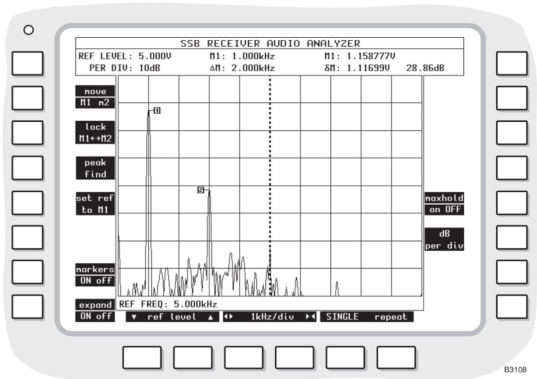
Fig. 3-24 SSB RECEIVER AUDIO ANALYZER expanded display with markers
