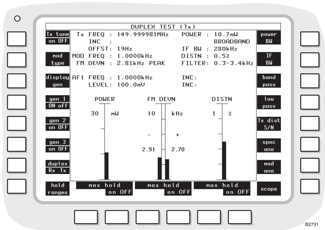
Fig. 3-15 DUPLEX TEST (Tx) display with bar charts
