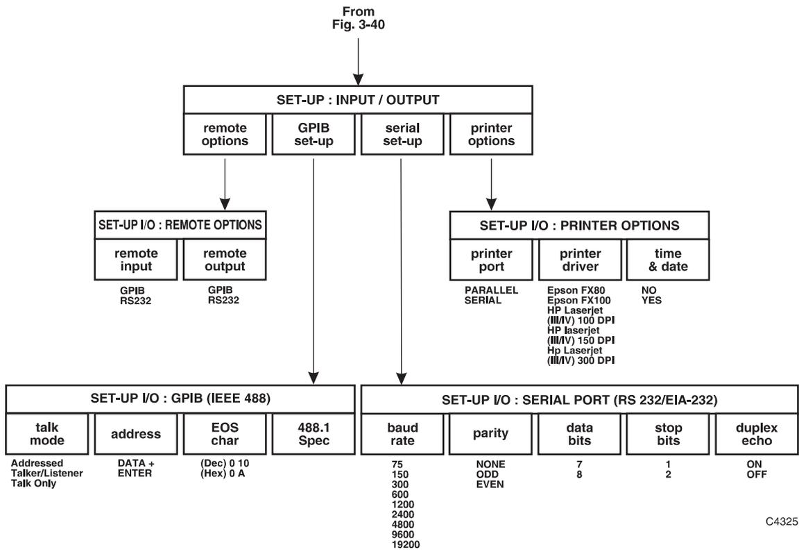
Fig. 3-43 HELP AND SET-UP - input/output
