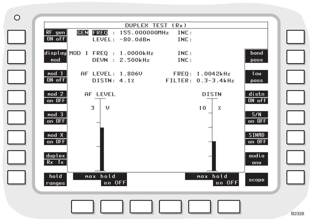
Fig. 3-16 DUPLEX TEST (Rx) display with bar charts
