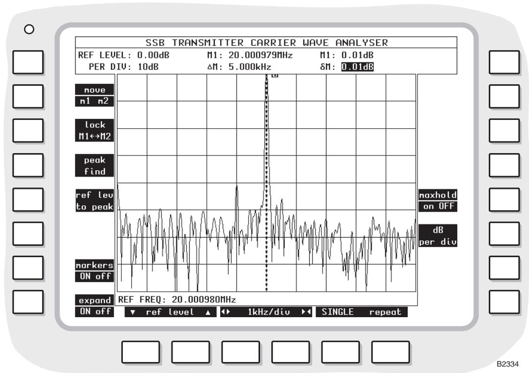
Fig. 3-22 SSB TRANSMITTER CARRIER WAVE ANALYZER expanded display
