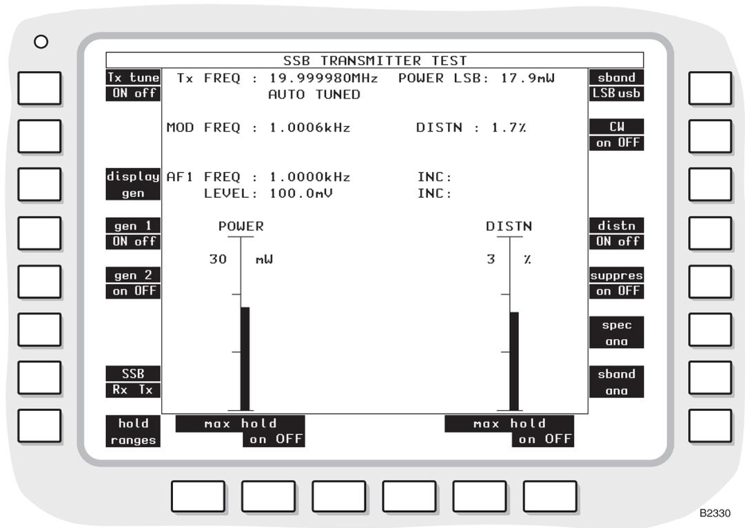
Fig. 3-18 SSB TRANSMITTER TEST display with bar charts
