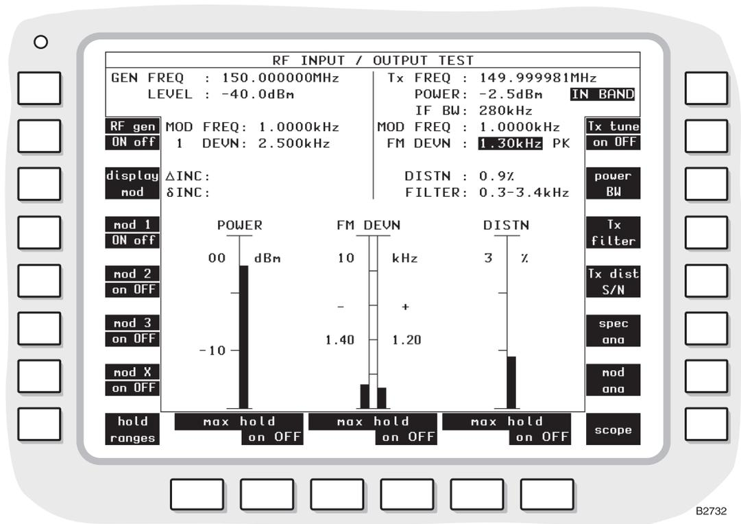
Fig. 3-17 RF INPUT/OUTPUT TEST display with bar charts
