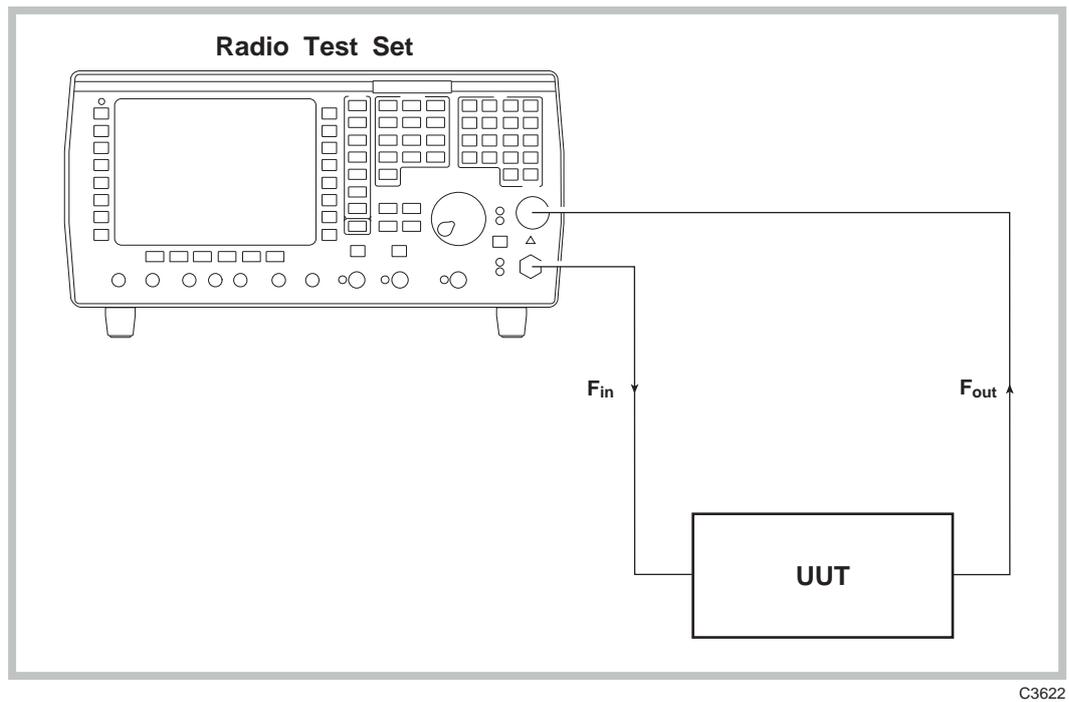
Fig. 3-52 Normal, doubler and divider testing
