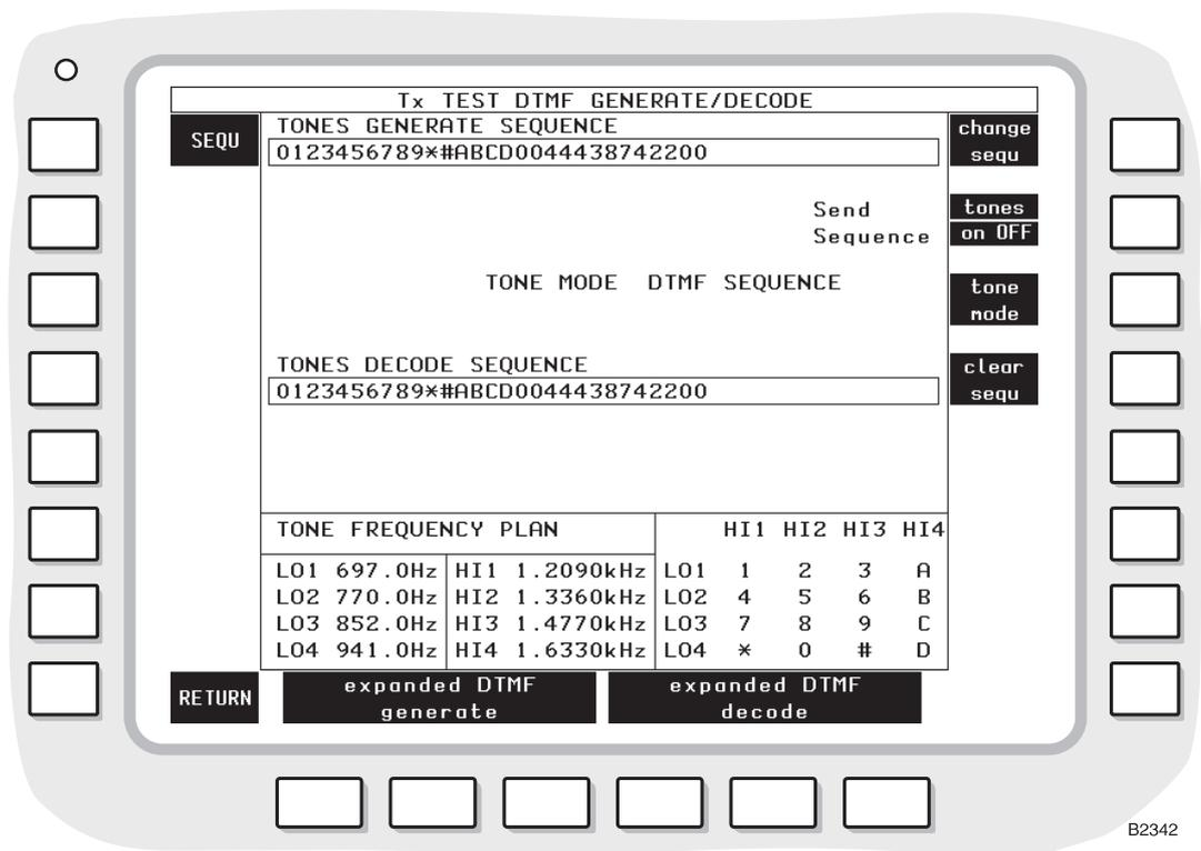
Fig. 3-32 Tx TEST DTMF GENERATE/DECODE display
