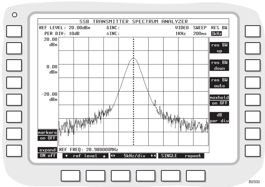
Fig. 3-20 SSB TRANSMITTER TEST SPECTRUM ANALYZER expanded display
