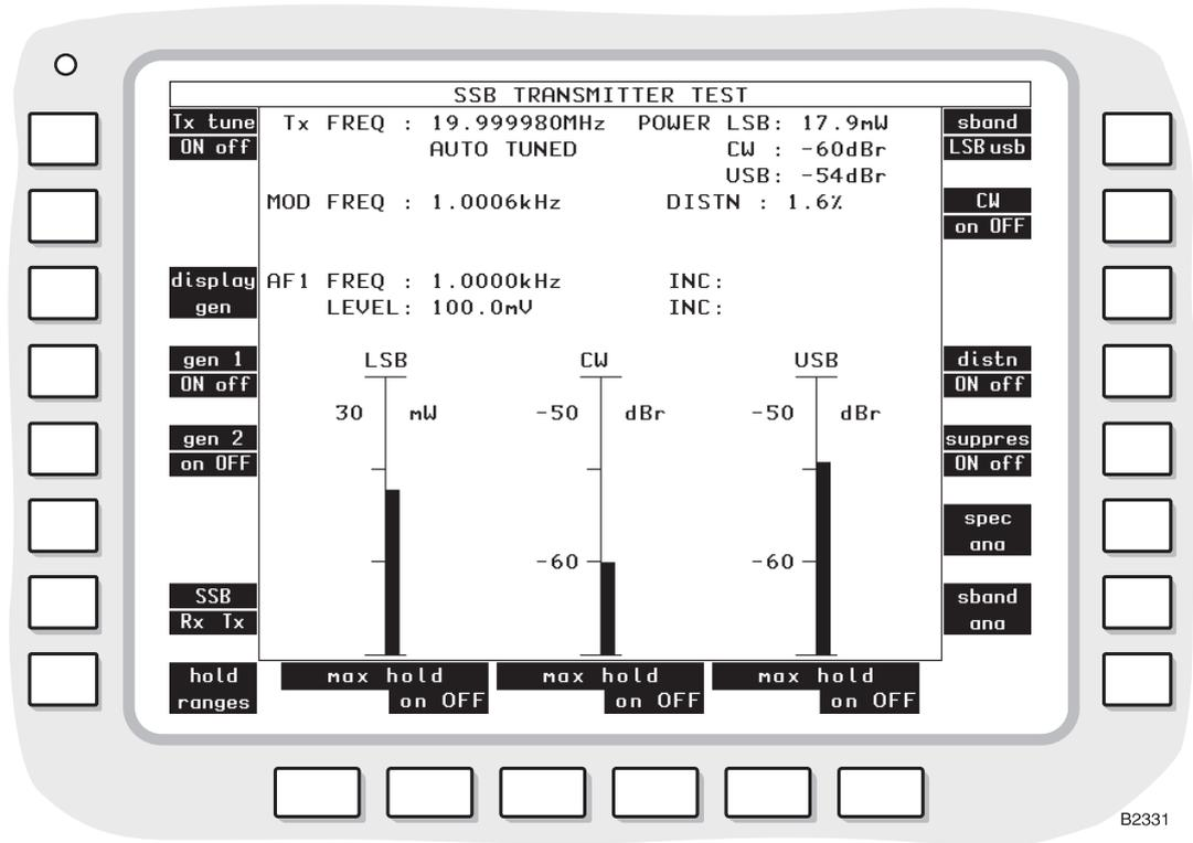
Fig. 3-19 SSB TRANSMITTER TEST display with suppression analyzer
