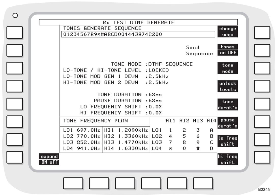
Fig. 3-35 Rx TEST DTMF GENERATE display
