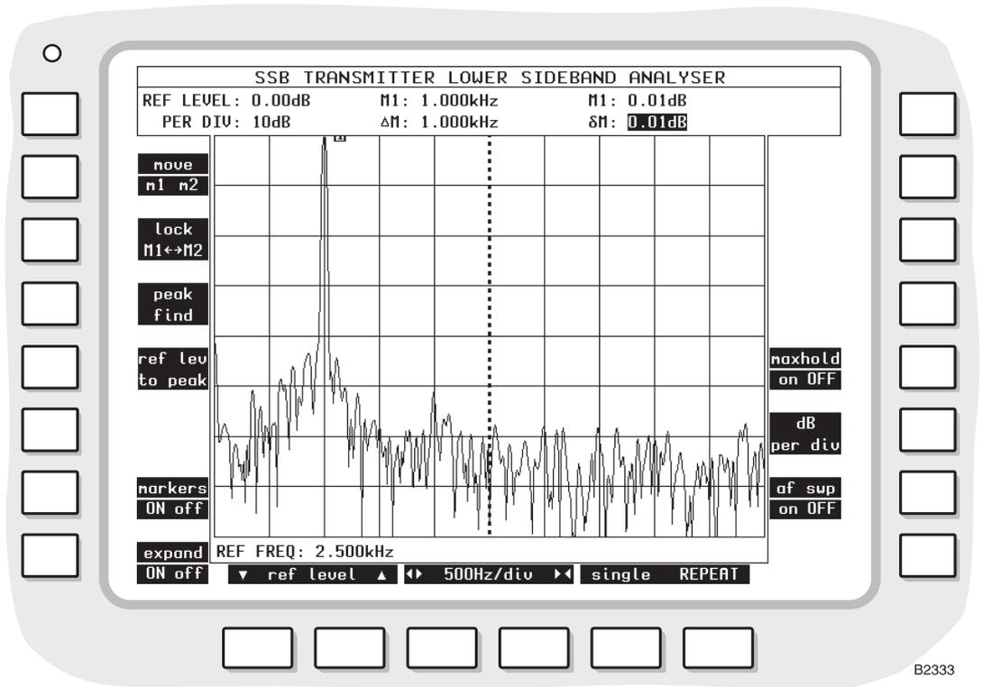
Fig. 3-21 SSB Transmitter Lower Sideband Analyzer expanded display with markers
