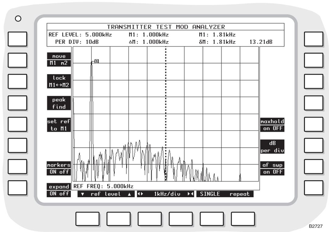
Fig. 3-9 TRANSMITTER TEST MOD ANALYZER expanded display with markers
