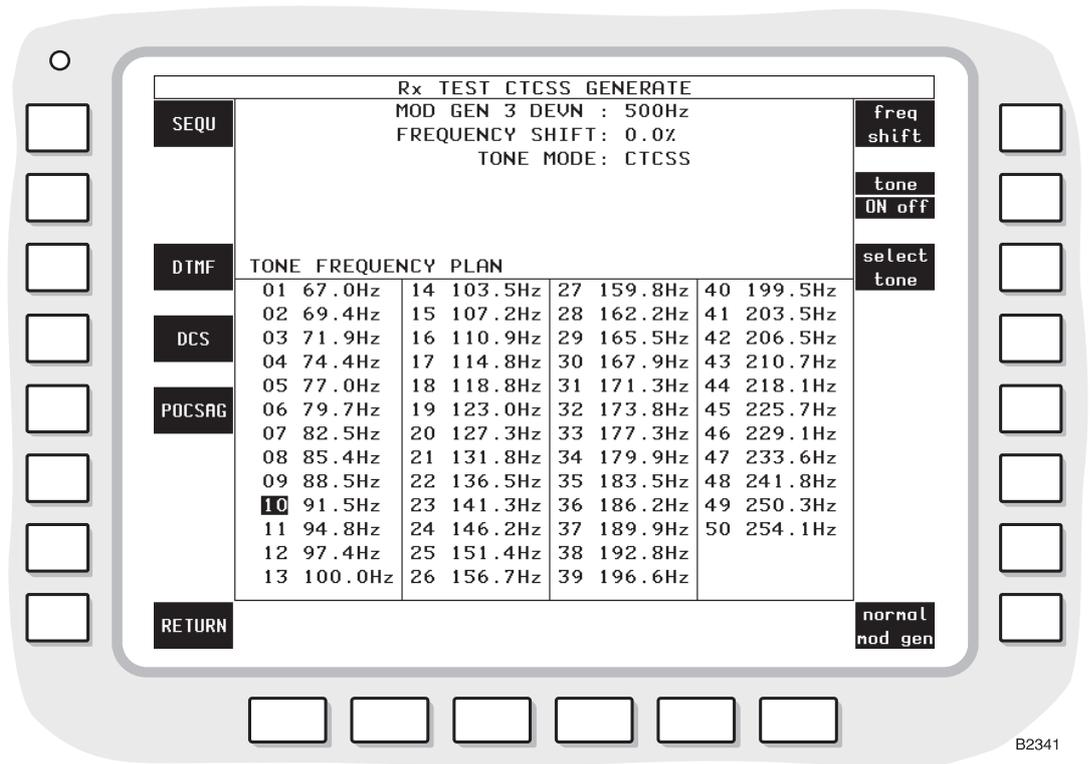
Fig. 3-30 Rx TEST CTCSS GENERATE display
