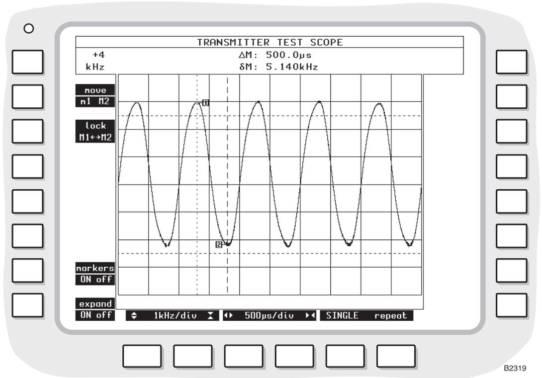
Fig. 3-7 TRANSMITTER TEST SCOPE expanded display with markers
