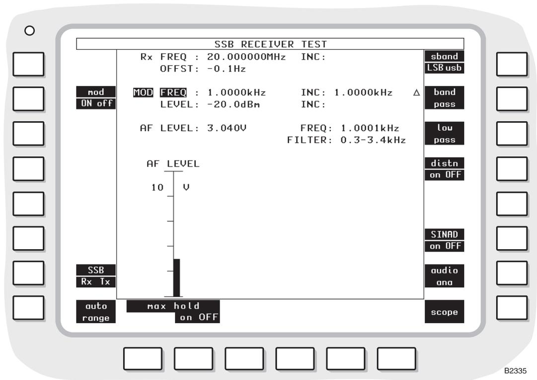
Fig. 3-23 SSB RECEIVER TEST display with bar charts
