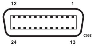
Fig. 2-1 GPIB socket contacts (as seen facing panel)
