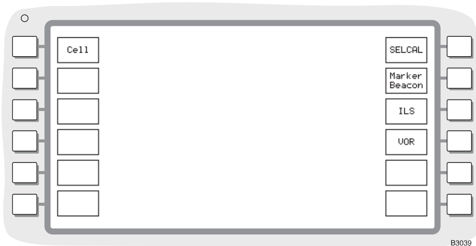
Fig. 2-2 Avionics/Cellular or Trunked system selection screen
