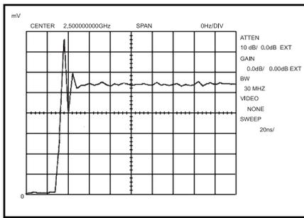
200 ns sweep clearly shows ringing on demodulated radar pulse
