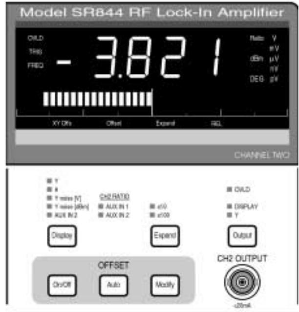
**Display** This key selects the Channel 2 Display quantity. Channel 2 may display Y [Volts],  $\theta$  [Degrees], Ynoise [Volts], Ynoise [dBm], or AUX IN 2 [Volts]. The displayed quantity appears on a 4½ digit display and also on the accompanying bar-graph display. An indicator shows the currently displayed quantity.
