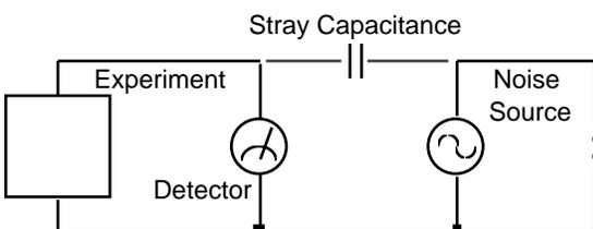
We can estimate the noise current caused by a stray capacitance by,
