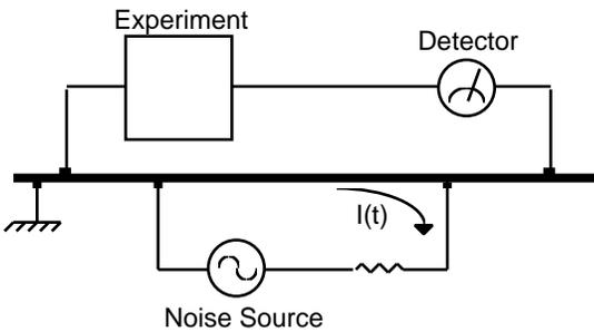
problem with reference frequency ground currents. In this illustration, the detector is measuring the signal relative to a ground far from the rest of the experiment. The experiment senses the detector signal plus the voltage due to the noise source's ground return current passing through the finite resistance of the ground between the experiment and the detector. The detector and the experiment are grounded at different places which, in this case, are at different potentials.
