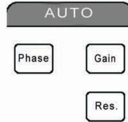
Pressing an Auto Function key initiates an auto function which may take some time. The AUTO leds in the CH1 and CH2 displays will be on while the function is in progress. A multi-tone sound will indicate when the auto function is complete and the AUTO leds will turn off.
