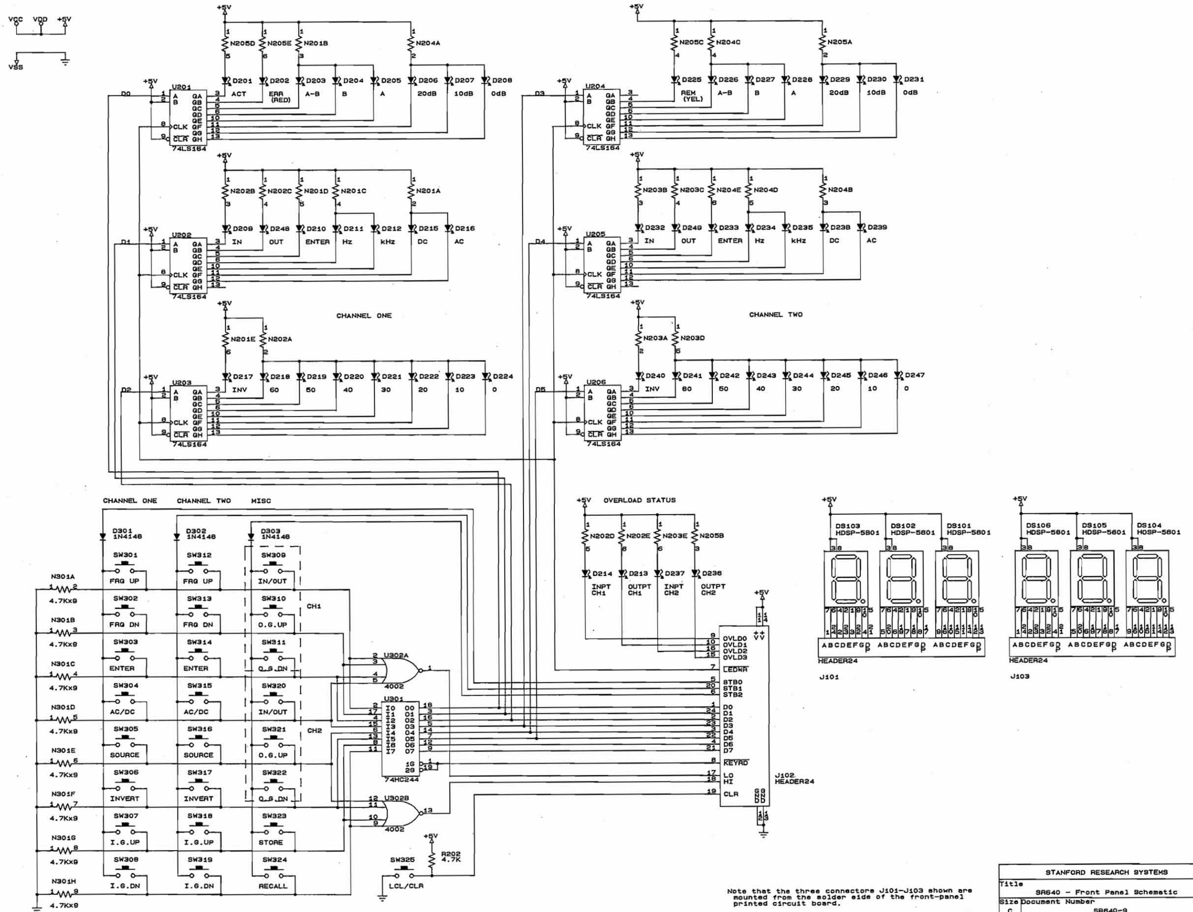
Note that the three connectors J101-J103 shown are mounted from the solder side of the front-panel printed circuit board.
