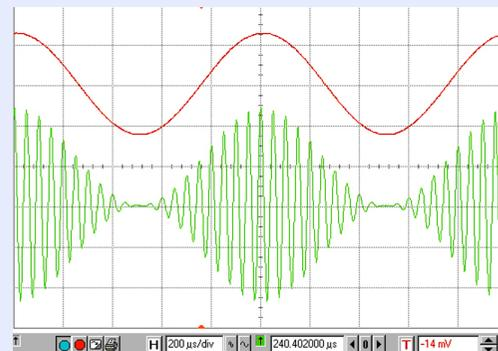
The frequency range of the SG380 Series extends from DC to 2 GHz, 4 GHz or 6 GHz (depending on model). All of the analog modulation modes also extend to DC allowing your SG380 to perform function generator tasks. Shown here is a 20 kHz carrier being amplitude modulated by a 1 kHz sine.
