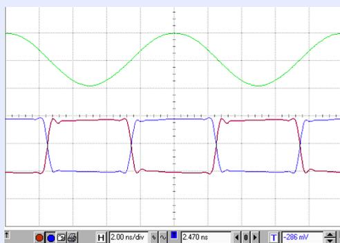
Option 01 provides differential clock outputs in addition to sine outputs. The clocks have transition times of about 35 ps. Both the offset and amplitude of the clock outputs can be adjusted for compliance with standard logic levels. Shown here at 2 ns/division: 100 MHz front-panel sine wave output (top trace) and differential clock outputs (bottom traces). The displayed transition times are limited by the 1.5 GHz bandwidth of the oscilloscope.
