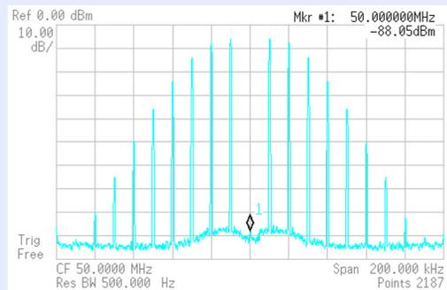
Outputs below 62.5 MHz are generated by direct-digital synthesis with a sample frequency of 1 GHz. In this example, a 50 MHz carrier is frequency modulated at a rate of 10 kHz and a deviation of 24.0477 kHz, for a modulation index  $\beta = 2.40477$ . The carrier amplitude is proportional to the Bessel function  $J_0(\beta)$ , which has its first zero at 2.40477.
