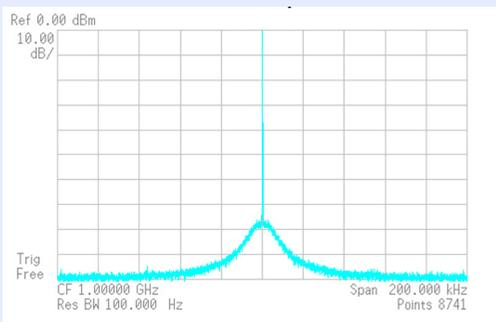
The SG380 Series outputs exhibit low phase noise and low spurious content. In this direct measurement taken with 100 Hz RBW, the noise floor of the spectrum analyzer dominates over most of the 200 kHz span.
