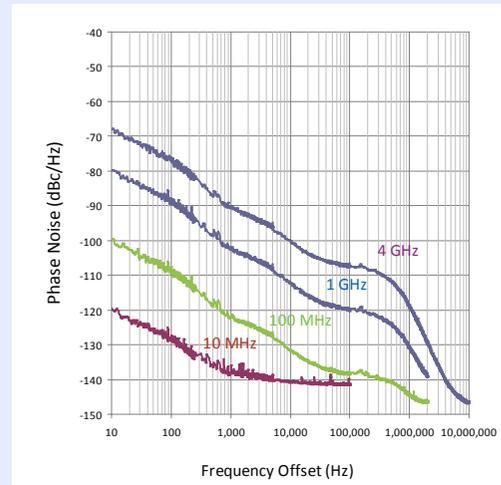
The SG380 Series always synthesizes a frequency in the top octave and digitally divides to generate outputs at lower frequencies. Doing so creates phase noise characteristics which scale with output frequency by 6 dB/octave or 20 dB/decade.
