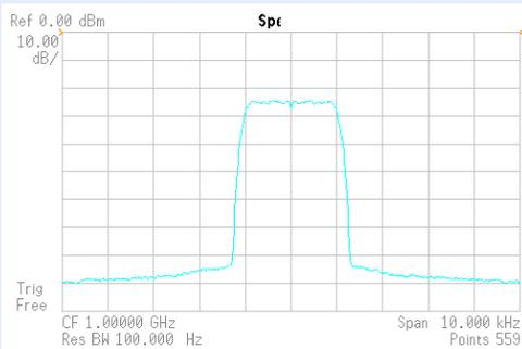
Option 03 allows I/Q modulation of carriers from 400 MHz to the upper frequency limit of your instrument. Two signal sources may be used for I/Q modulation: external I & Q inputs or an internal noise generator. The external I & Q BNC inputs are on the rear panel. The internal noise generator has adjustable noise bandwidth. Shown here is a 1 GHz carrier being modulated by the internal noise generator with 1 kHz noise bandwidth.
