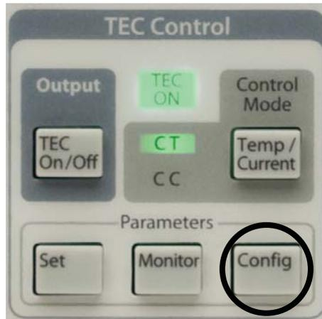
Figure 3.7: The TEC configuration menu selection.
