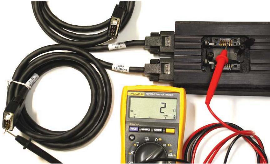
Figure 2.4: Verifying correct wiring prior to use.
