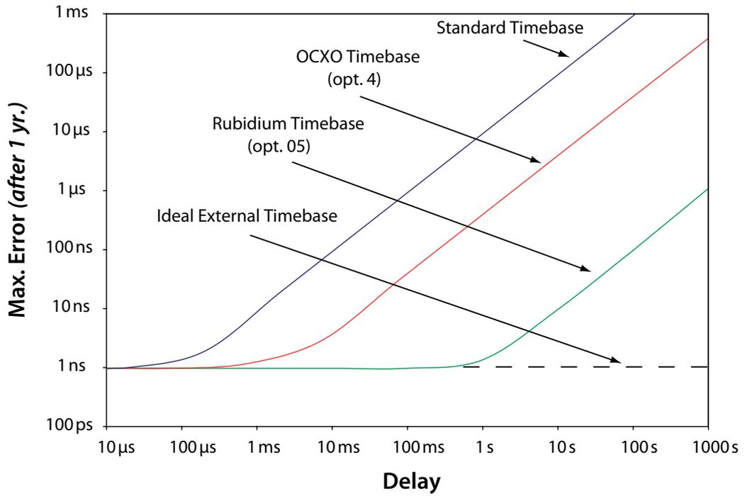
Figure 2: Typical DG645 Timing Error 1 Year after Calibration
