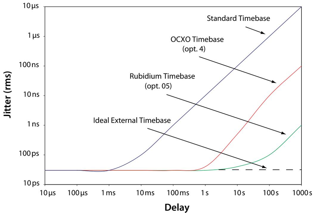
Figure 3: Typical rms Jitter vs. Delay Setting
