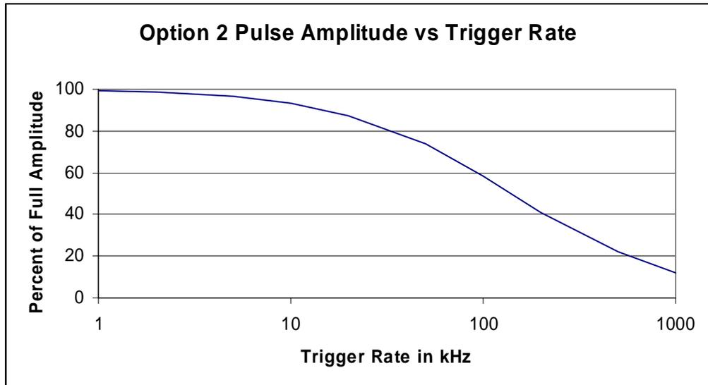
**Figure 6: Option 2 Amplitude Reduction vs. Trigger Rate**
