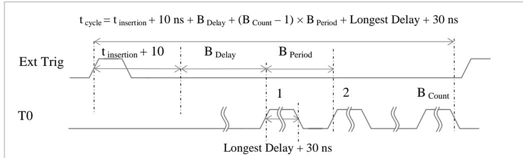
**Figure 14: Burst Timing**
