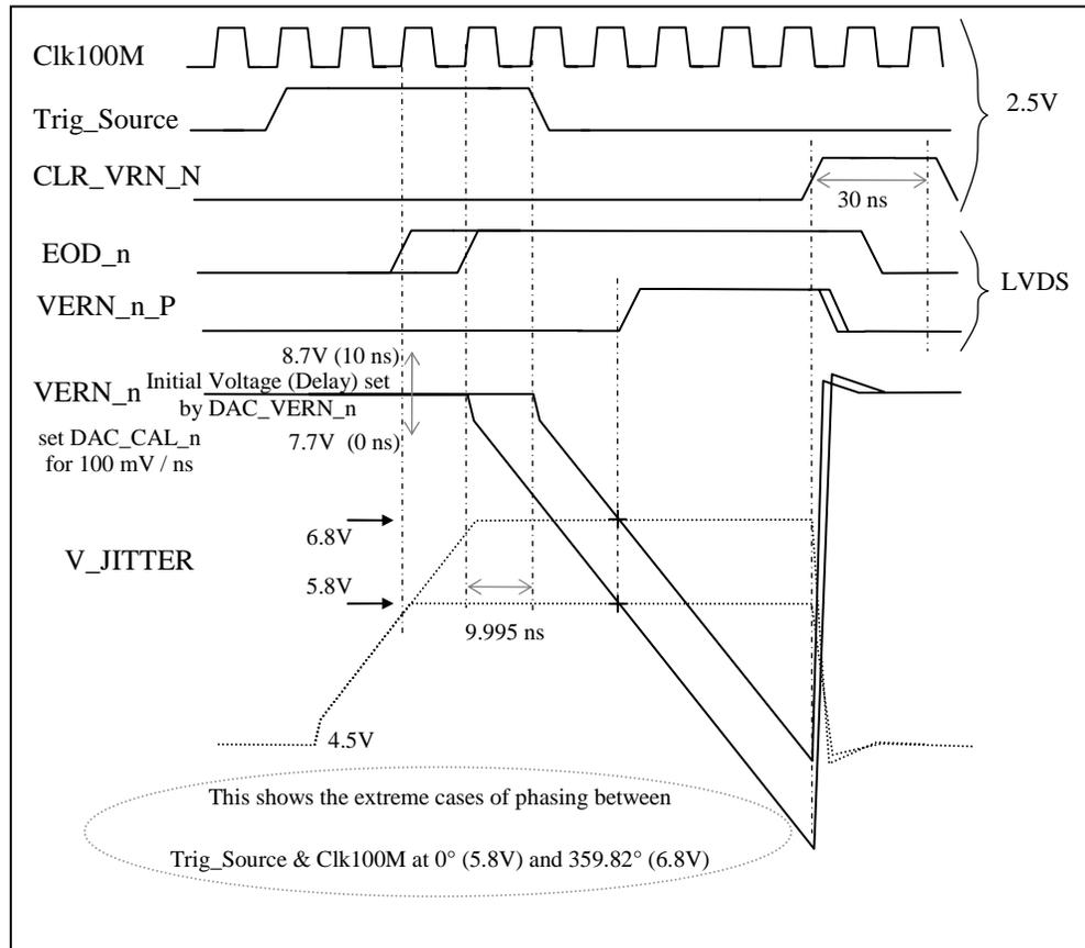
Figure 16: Vernier Waveforms
