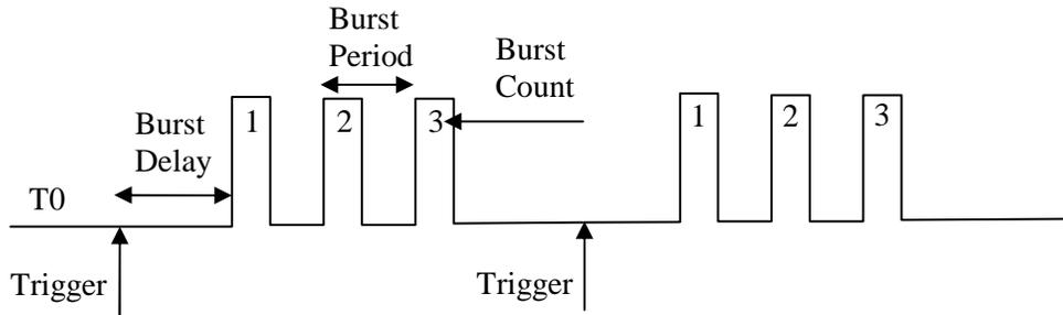
Figure 11: T<sub>0</sub> Output in Burst Mode
