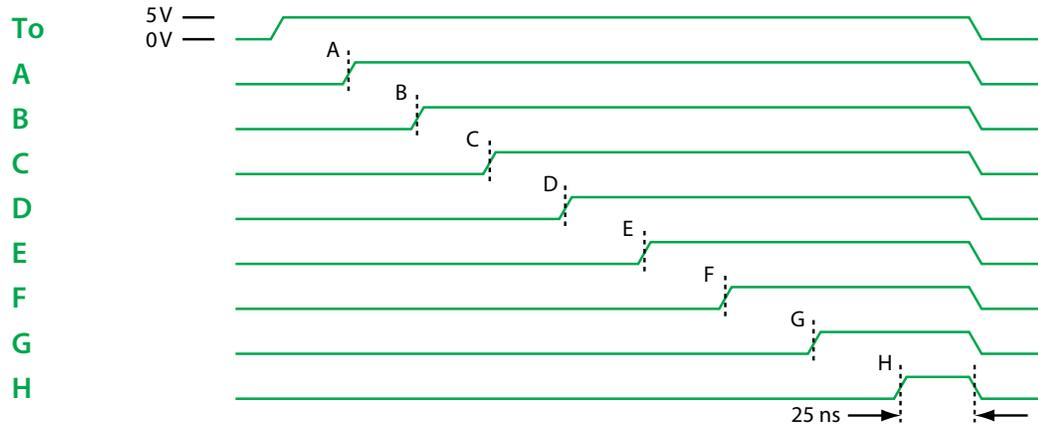
Figure 4: Option 1 Rear-Panel Outputs vs. Programmed Delay
