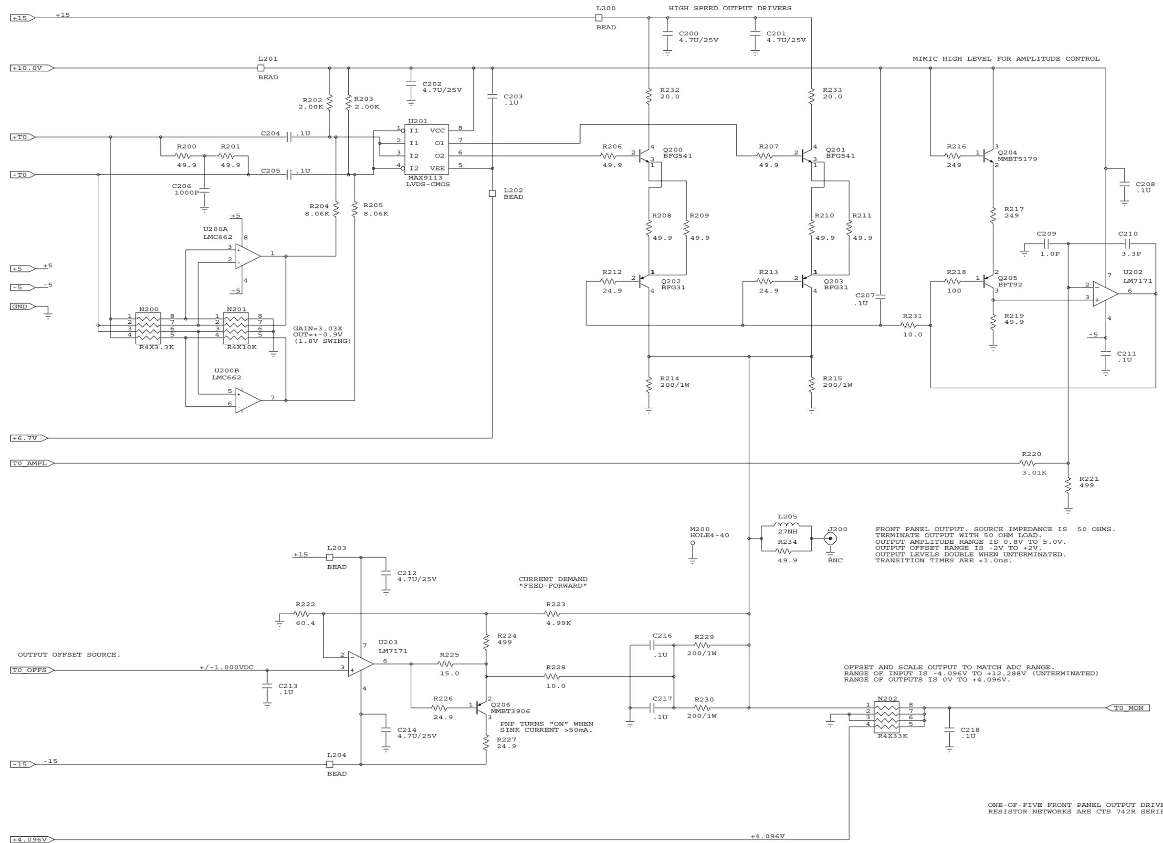
FRONT PANEL OUTPUT. SOURCE IMPEDANCE IS 50 OHMS.
