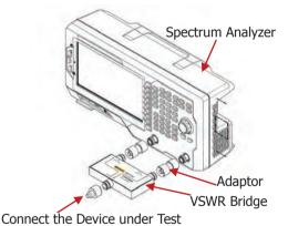
Connect the device under test
