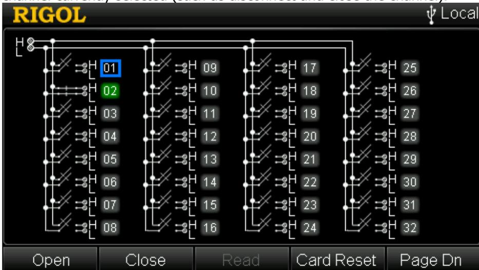
Figure 2-18 MC3132 Control Interface (Bank Joined)
