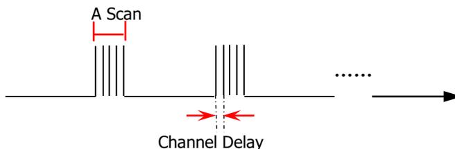
When the current channel is a multiplexer channel, enter the fourth step of the channel configuration guide, use the up/down direction key to select **Delay** and use the left/right direction key to select "Auto" or set a specific delay value.
