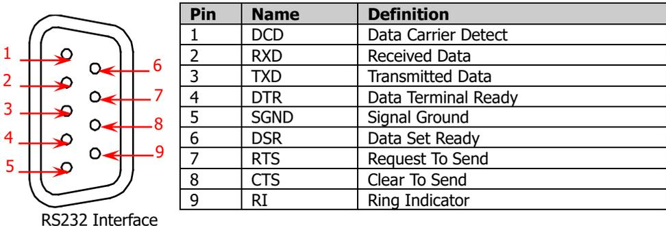
Connect the RS232 interface with the PC or data terminal equipment (DTE) device using a RS232 cable and set the interface parameters (such as the baud rate and parity) to match the PC or terminal device. At this point, you can control the instrument remotely. The measurement result of the instrument can be output to serial port receiving devices via this interface.
