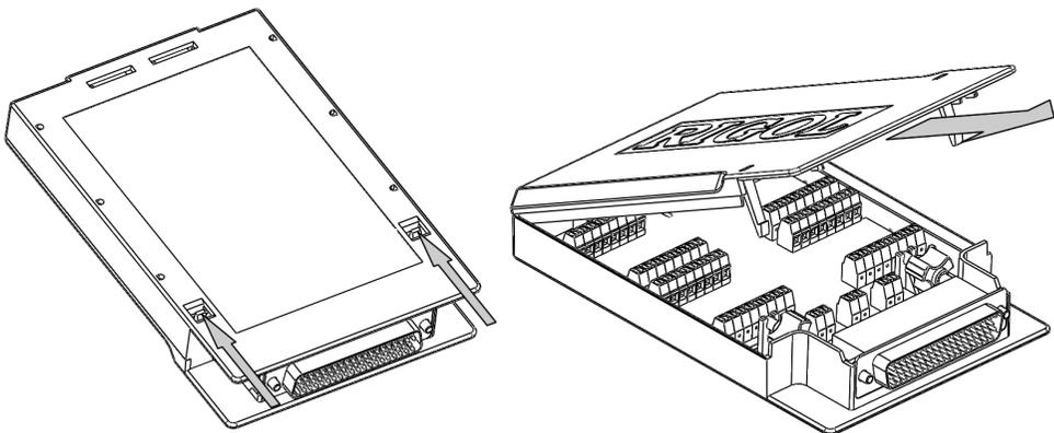
2. Connect the cables for connecting the signal under test according to the labels on the circuit board of the terminal block (for the connecting method, refer to Table 1-2). Pass the binding wires through the two groups of holes as pointed out by the arrows in the figure below to fix the cable connected. Pay attention
