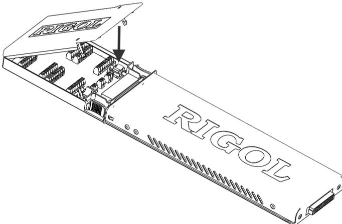
5. Insert the module with the terminal block into the slot of the mainframe.
