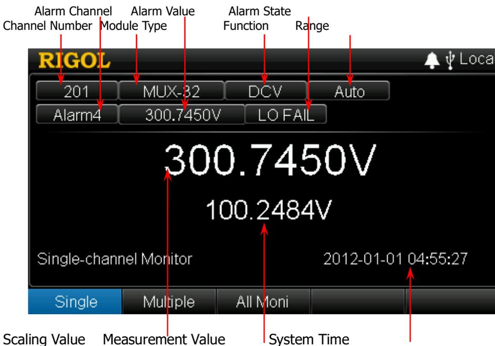
Figure 2-12 Single-channel Monitor
