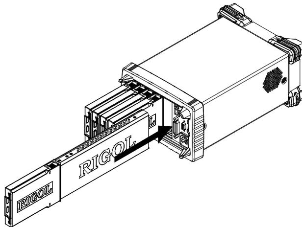
Figure 1-8 Insert the Module into the Mainframe
