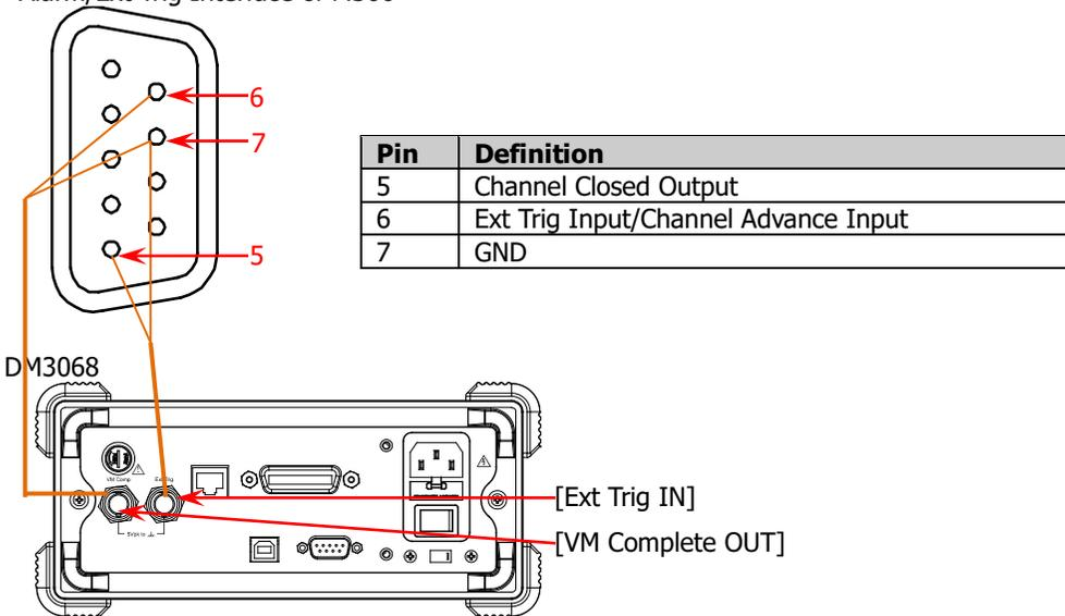
Figure 3-1 To Connect External DMM Schematic Diagram
