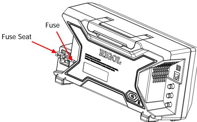
Figure 1-16 To Replace the Fuse
