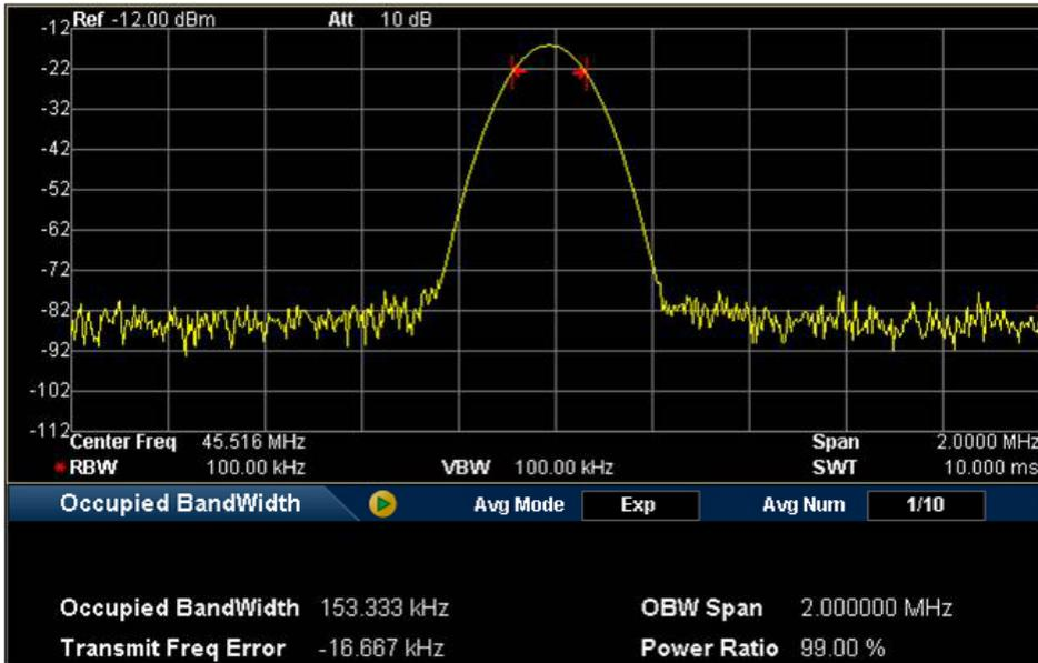
Figure 2-17 OBW Measurement Interface
