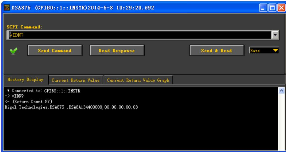
Figure 3-9 Write and Read Commands via GPIB
