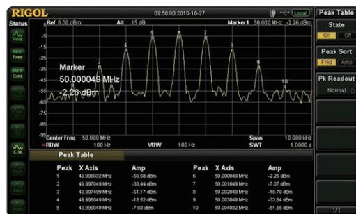
The advanced Harmonic distortion measurement function
