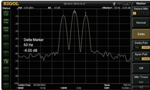
Readout the signal's Phase Noise directly by using the standard Noise Marker function
