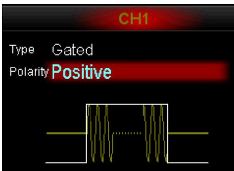
Gated Burst could only be triggered by "External" source. You can also set "Start Phase".
