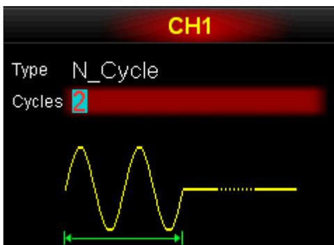
N Cycle Burst could be triggered by "Internal", "External" or "Manual" source. You can also set "**Start Phase**", "**Burst Period**" (internal trigger), "**Delay**", "**Trigger Input**" (external trigger) and "**Trigger Output**" (internal and manual triggers).
