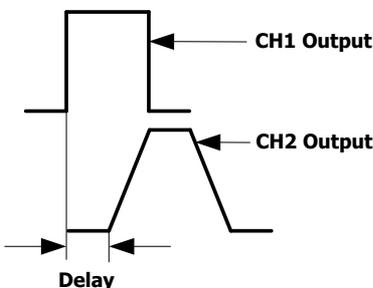
Press **Pulse** → **Delay** to highlight the softkey, and then use the numeric keyboard to
