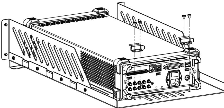
5. Install the Front Panel: aiming the instrument front panel at the opening of the Front Panel of the machine rack and fix them with four M4 screws.
