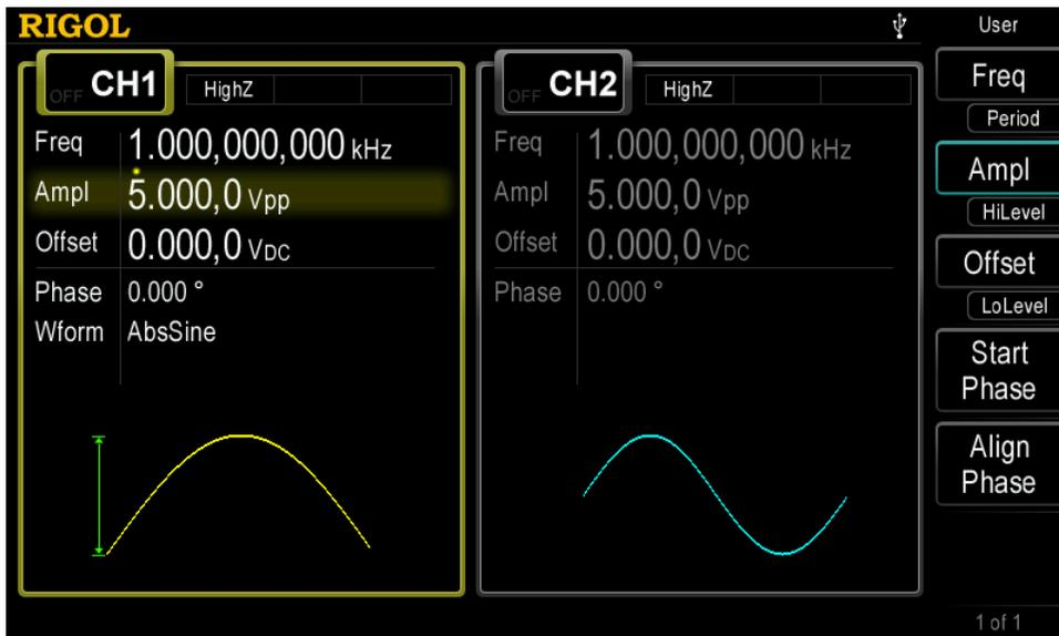
Figure 10-6 Press **User** to Quickly Recall the Waveform
