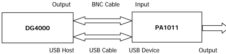
After DG4000 and PA1011 are successfully connected as shown in the figure above, press **Utility** → **PA Set** to open the parameter setting interface of the power amplifier.
