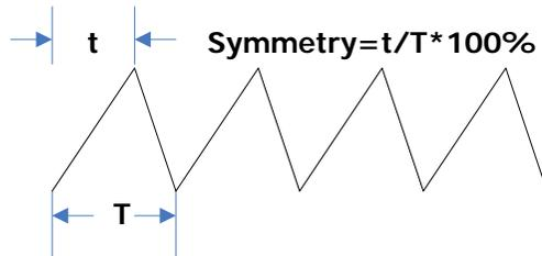
The setting range of symmetry is from 0% to 100% and the default is 50%.
