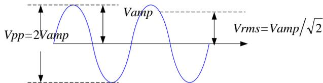
According to the figure above, the conversion relation between Vpp and Vrms fulfills the following equation.
