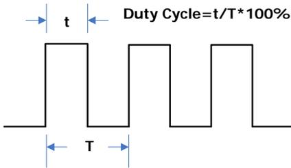
The duty cycle range is limited by the "**Freq/Period**" setting. Please refer to "Signal Characteristics" in "**Specifications**". The default value is 50%.
