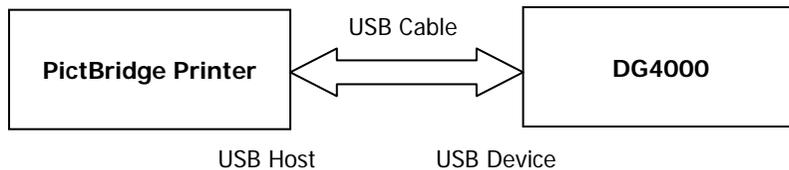
Press **Utility** → **I/O Config** → **USB Dev** to set the device type to "Printer". Press **Utility** → **Print Set** → **Dest** to select "Printer". Then, press **Printer Set** to enter the print setting menu.
