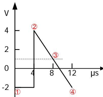
**Explanation:** As can be seen from the above figure, the waveform editor inserts values at the start point (point 2) and the stop point (point 4) according to the current interpolation mode; then, it automatically generates point 1 and point 3 to create a continuous waveform.
