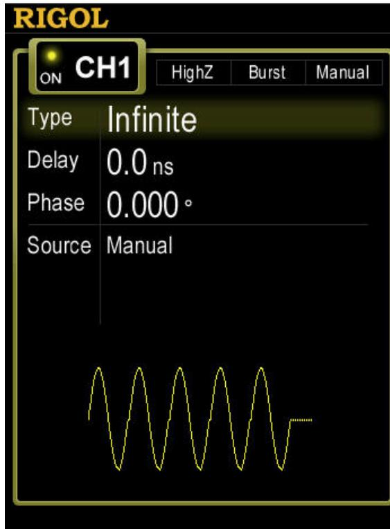
Figure 7-2 Infinite Burst
