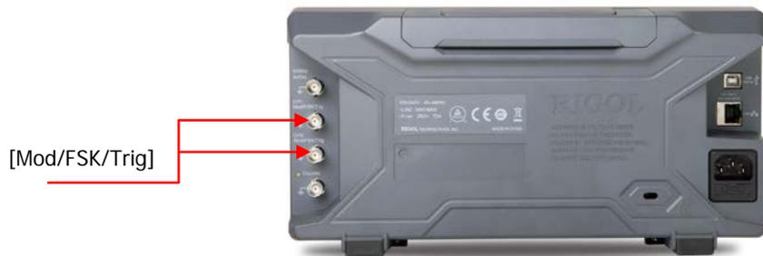
Note: The **[Mod/FSK/Trig]** connector is different when controlling ASK and AM/FM/PM modulations externally. In ASK modulation, the **[Mod/FSK/Trig]** connector has adjustable edge polarity.
