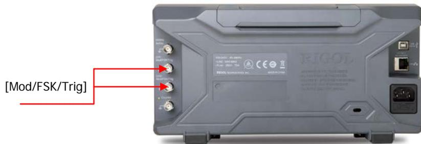
Note: The **[Mod/FSK/Trig]** connector is different when controlling PSK and AM/FM/PM modulations externally. In PSK modulation, the **[Mod/FSK/Trig]** connector has adjustable edge polarity.
