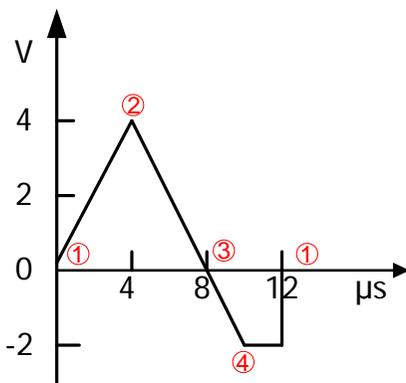
**Explanation:** As can be seen from the above figure, the waveform editor always connects the voltage levels of the first point to the last point in sequence and then hold this level until the cycle period expires to create a continuous waveform.
