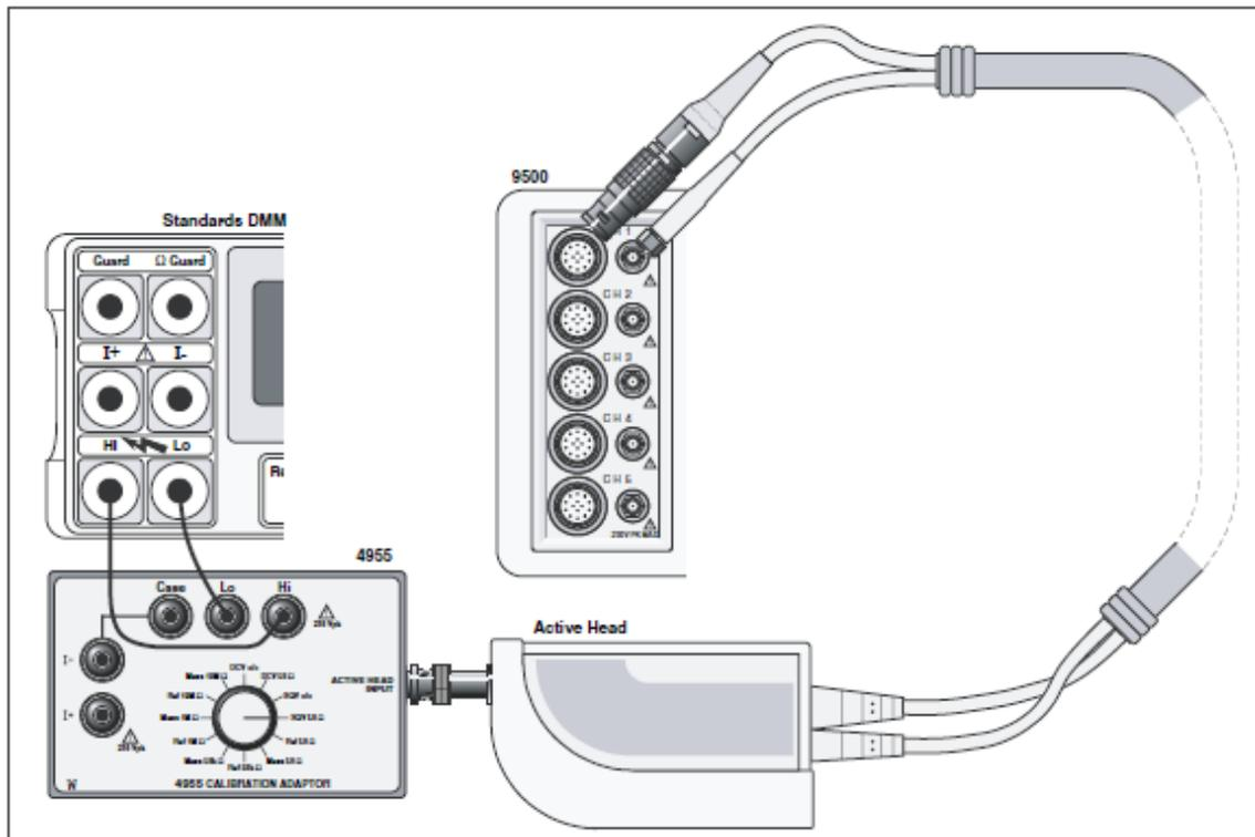
Figure 5. LF Sine Voltage Verification — Interconnections
