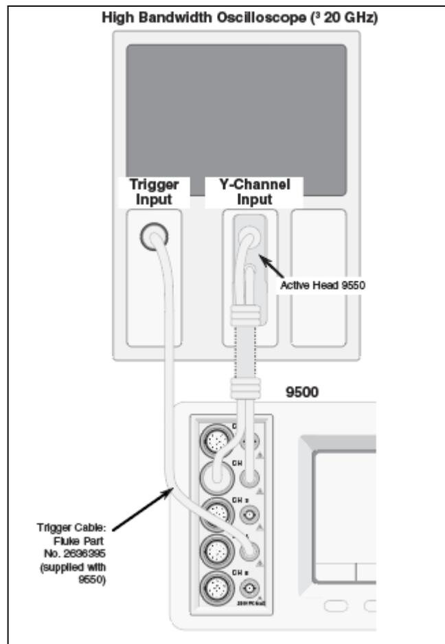
**Figure 21. 25 ps Edge Function Calibration — Interconnections**
