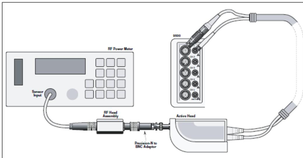
Figure 19. RF Sine Voltage Calibration — Interconnections
