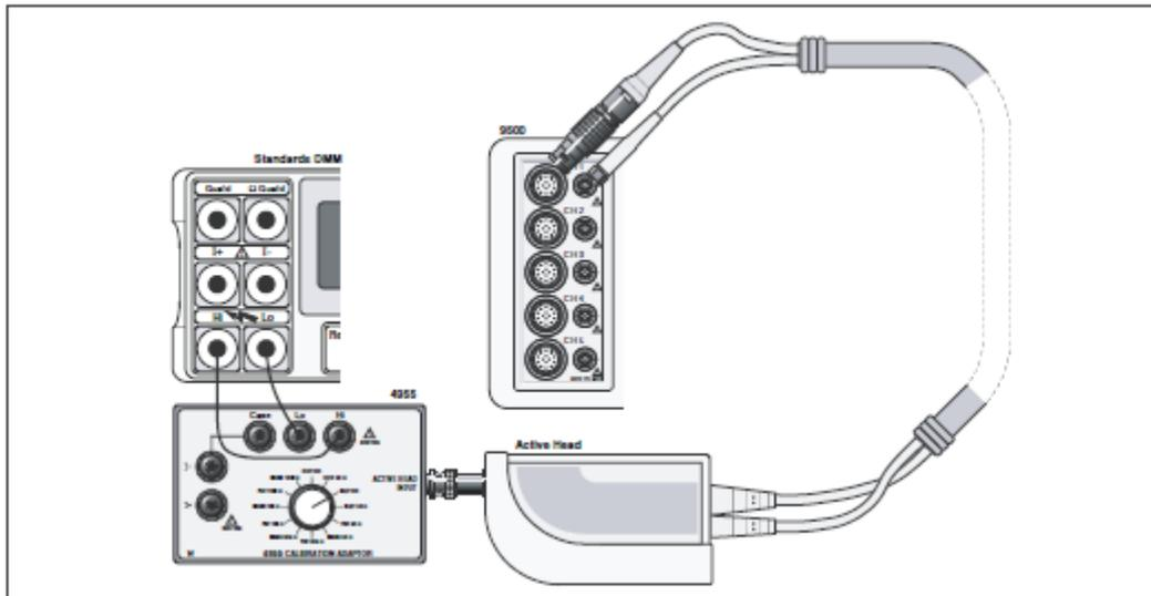
Figure 18. LF Sine Voltage Calibration — Interconnections
