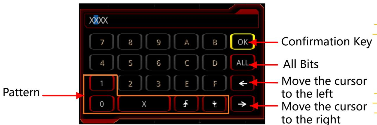
**Figure 8.6 Virtual Keypad for Pattern Setting**
