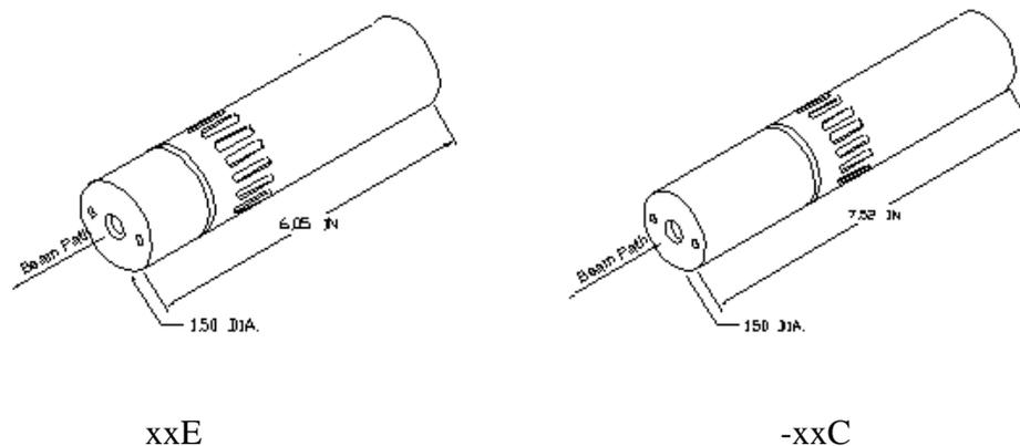
Figure 1 Dimensions of LQx and RLx series
