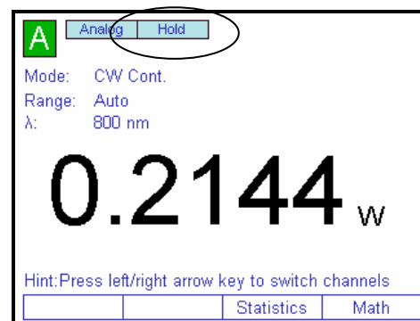
Figure 37 Measurement is on hold
