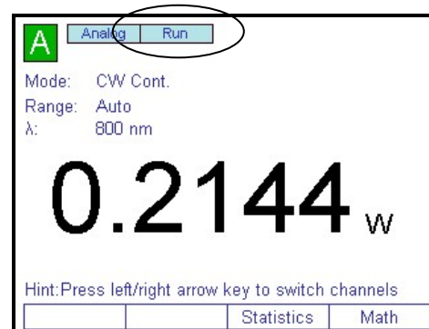
Figure 38 Measurement is running
