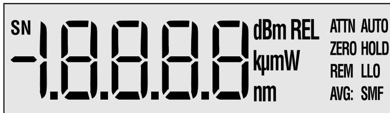
Figure 5. The 1830-C Liquid Crystal Display
