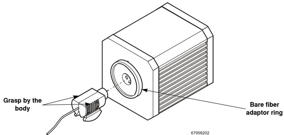
Figure 2.11 Inserting the BF-820
