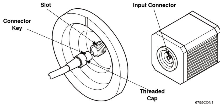
**Figure 2.5** Connecting an FC/PC Bulkhead Patch cord
