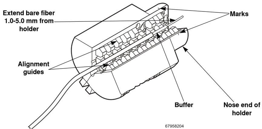
Figure 2.9 Place Fiber in BF-820 Fiber Holder
