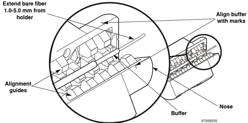
Figure 2.10 Place Fiber in BF-820 Fiber Holder
