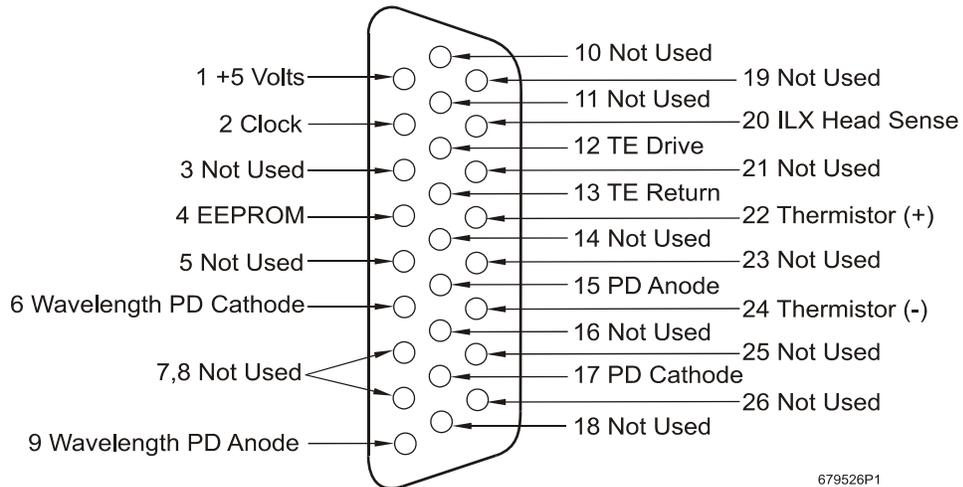
Figure 2.1 26-pin Input Connector Pin-out Diagram
