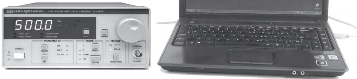
The USB interface allows for quick, effortless remote control for fast, repeatable instrument control during L-I testing and R&D or manufacturing control applications.
