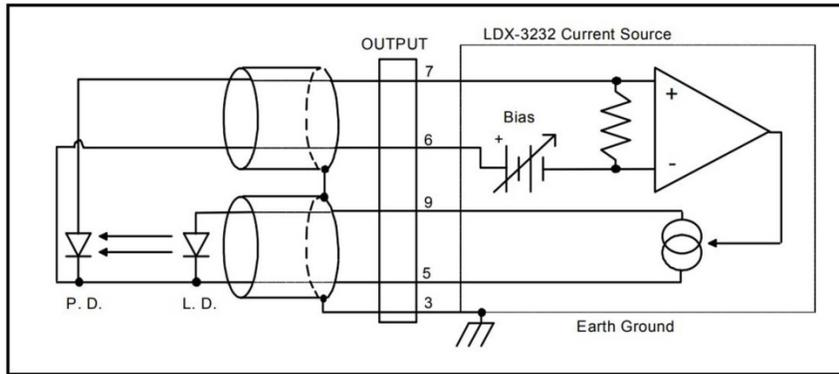
**Figure 2.1** Common Laser Cathode & Photodiode Cathode
