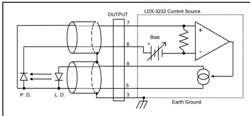
**Figure 2.2** Common Laser Cathode & Photodiode Anode
