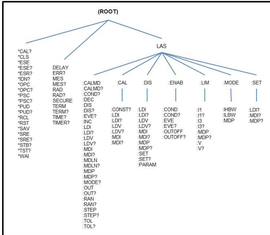
**Figure 3.1** LDX-3232 Command Path Structure
