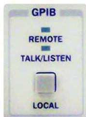
Sending a command over the GPIB automatically puts the instrument in REMOTE mode. The REMOTE indicator will identify when the Current Source is in remote operation mode. When the instrument is in REMOTE mode, pressing the LOCAL button returns the instrument to LOCAL control mode.
