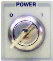
To turn on the LDX-3232, rotate the key in the POWER section of the front panel from O to I. This action will initiate the power on sequence. If the LDX-3232 does not appear to turn on, verify that it is connected to line power. If line power is not the problem, remove the power cord and check the voltage selection block in addition to the line power fuse.
