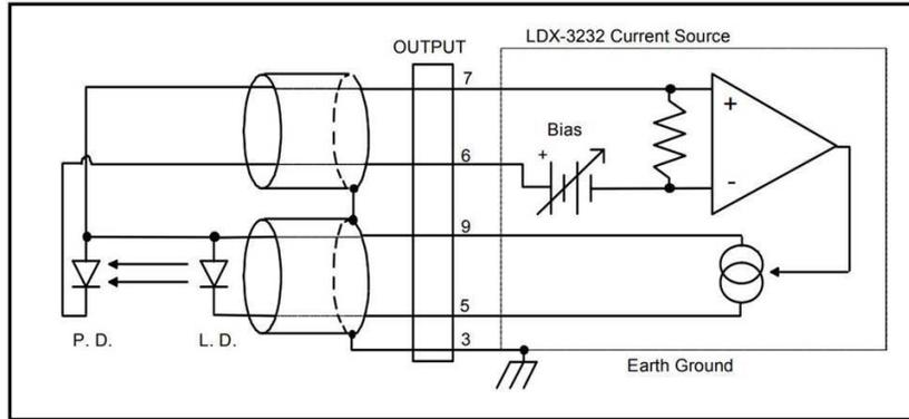
**Figure 2.4** Common Laser Anode & Photodiode Anode
