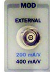
**Notes:** The limit clamp function for DC output current also applies to the modulated current, protecting the laser in any mode.
