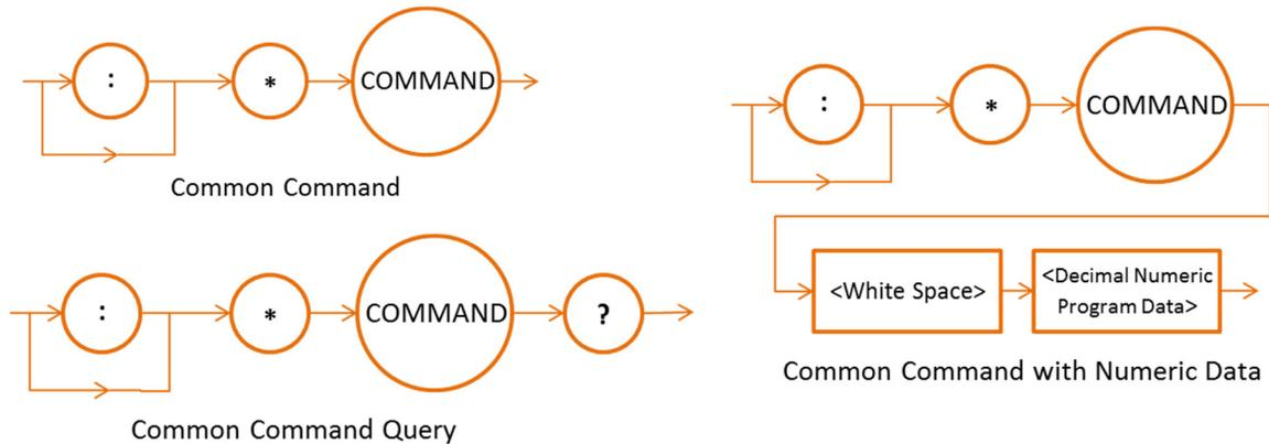
**Figure 3.2** Common Command Structure
