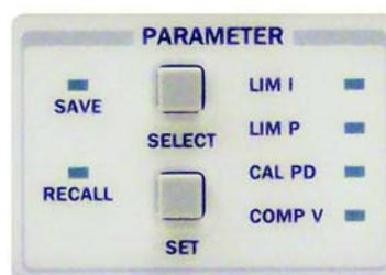
To adjust these values, press the (PARAMETER) SELECT button until the indicator next to the parameter which is to be adjusted is lit, then press the (PARAMETER) SET button. Adjust the value using the ADJUST KNOB. After three seconds, the new parameter value is stored in non-volatile memory.
