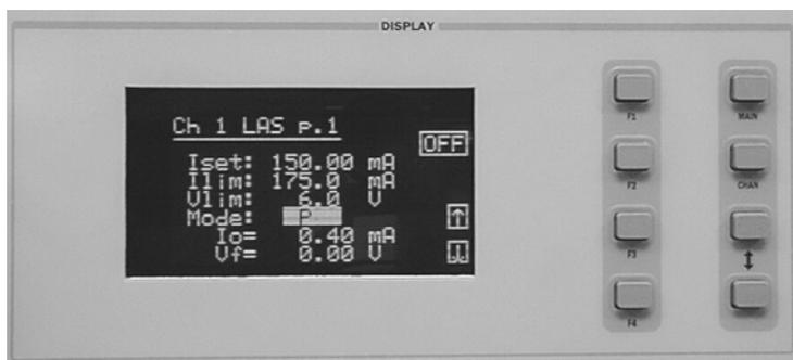
Select the Mode parameter by pushing the (DISPLAY) UP/DOWN ARROW keys until the Mode parameter is highlighted. Repeatedly pushing the (ADJUST) UP/DOWN ARROW keys or turning the ADJUST knob will cycle through the Constant Current low bandwidth (Ilbw), Constant Optical Power (P), Constant Current high bandwidth (Ihbw), and Photodiode Current (Ipd) control modes. Set the LDC-3916330 Series Controller Module in Constant Optical Power mode by selecting the P mode.
