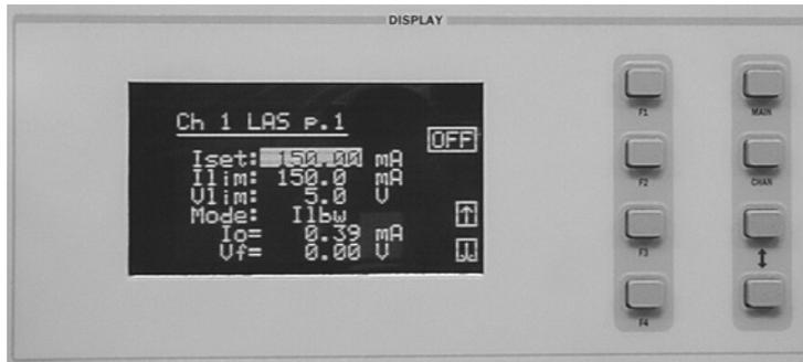
Next, select the Iset parameter on the setup menu using the (DISPLAY) UP/DOWN ARROW keys. This parameter sets the laser current source drive value when in Ilbw or Ilbw modes. Enter 150 mA using the numeric keypad, the ADJUST knob, or the (ADJUST) UP/DOWN ARROW keys. Push the ENTER key to store the value in memory within three seconds after entering the value using the numeric keypad, or it will revert to the old value.
