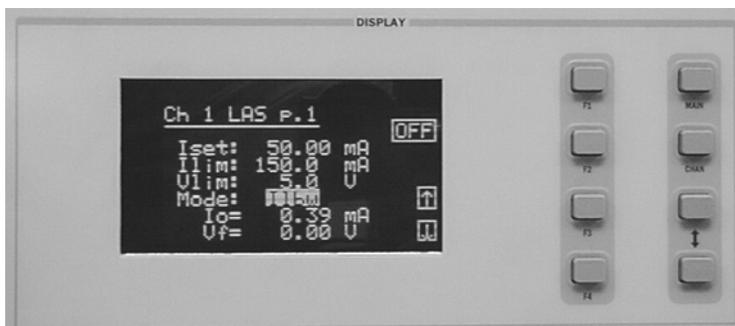
Select the Mode parameter by pushing the (DISPLAY) UP/DOWN ARROW keys until the Mode parameter is highlighted. Repeatedly pushing the (ADJUST) UP/DOWN ARROW keys or turning the ADJUST knob will cycle through the Constant Current low bandwidth (Ilbw), Constant Optical Power (P), Constant Current high bandwidth (Ihbw), and Photodiode Current (Ipd) control modes. Set the LDC-3916330 Series Controller Modules in Constant Current low bandwidth mode by selecting the Ilbw mode.
