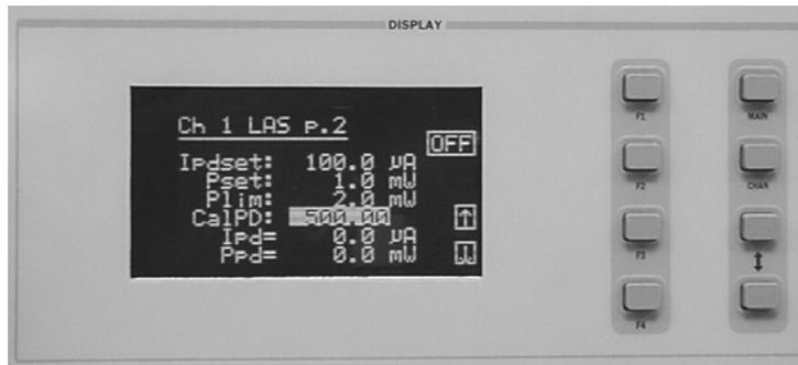
The correct responsivity value (CalPD) must be set for the constant power mode to operate properly. To do this, select the CalPD parameter, and adjust it to the correct value. The CalPD units are  $\mu\text{A}/\text{mW}$ .
