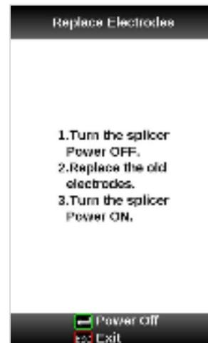
To remove and replace the electrodes:
