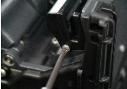
2. Clamp unit is made to slide and exchanged for other size.
