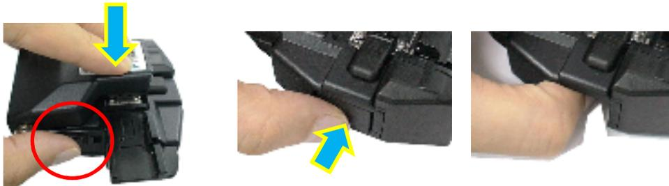
Press down the cutting lever. Release the pressure on the cutting lever. A spring force will bring it to its open position.
