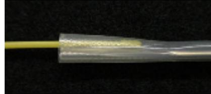
When a protection sleeve set position exceeds a yellow line, un-contracting of a protection sleeve occurs.
