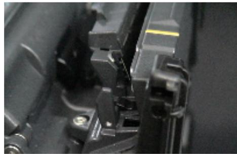
When using Fujikura Fuse Connect, removing the clamp is unnecessary.
