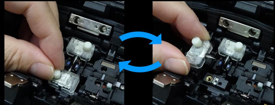
The transparent electrode covers support wider illumination of the v-groove. As the sheath clamp opens on the opposite side of the illumination lamp, the sheath clamp area is illuminated without shadow.
