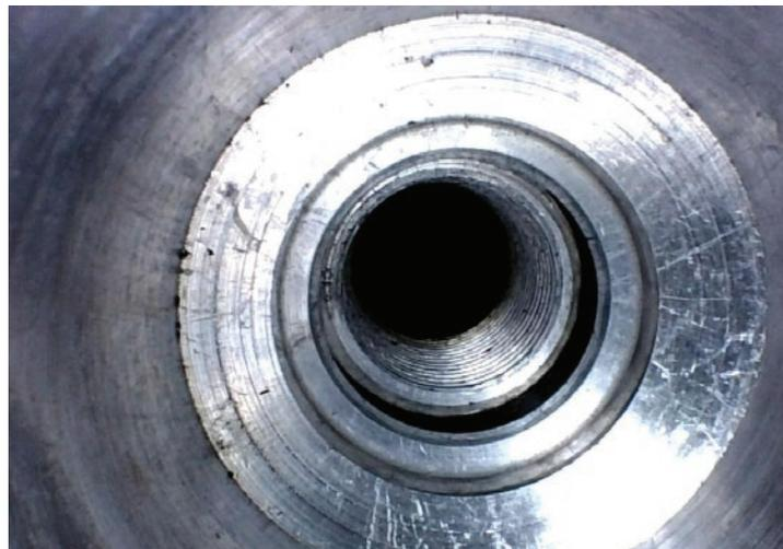
Photo above: Spark plug port inspection
