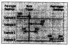
With Option -010, the burst memory may capture any group of 400 successive readings that occur within 399 readings prior to and 999 readings following the burst trigger. In example A, only one reading is taken after the trigger point. In example B, 400 readings immediately following the burst trigger are captured. Example C shows storage of 100 readings prior and 300 readings after the trigger point. The last example shows 400 readings being stored commencing 599 readings after the trigger.
