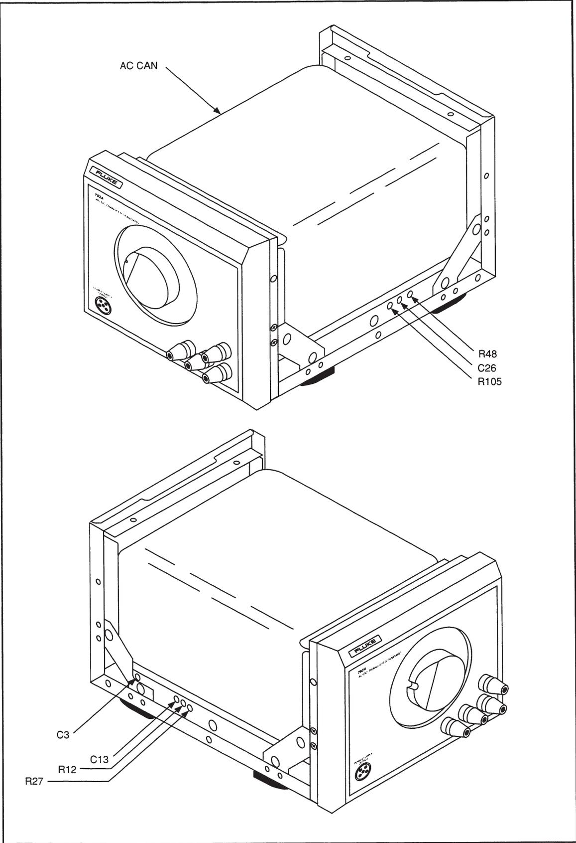
Figure 5-5. Location of Adjustments on the AC Plate
