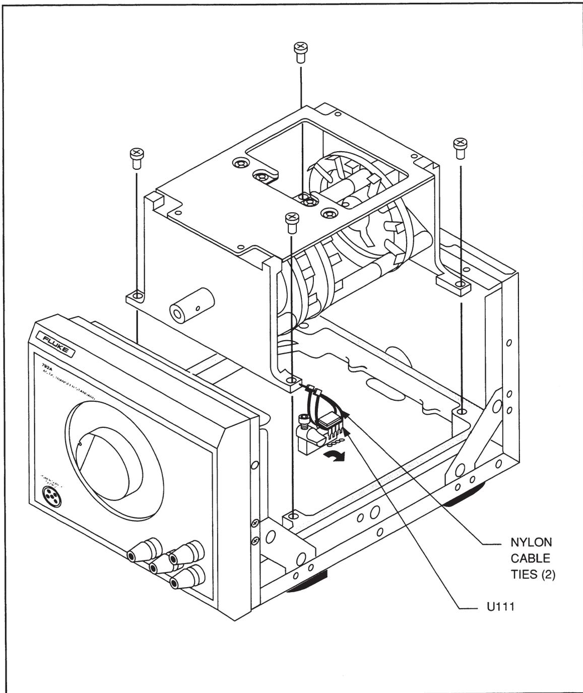
Figure 5-4. Replacing U11
