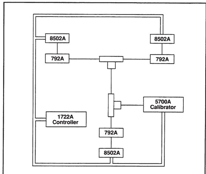
Figure 2. Block Diagram of the 792A Comparison System.
