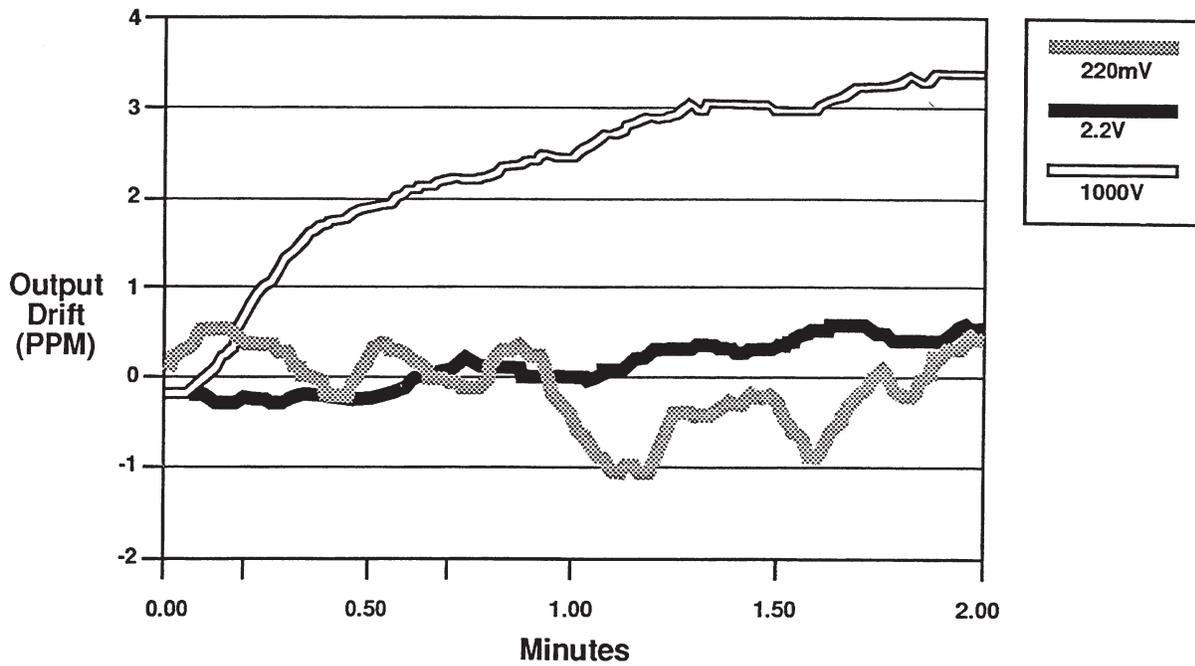
Figure 5. 792A Output Drift: 220 mV, 2.2 V & 1000 V Ranges
