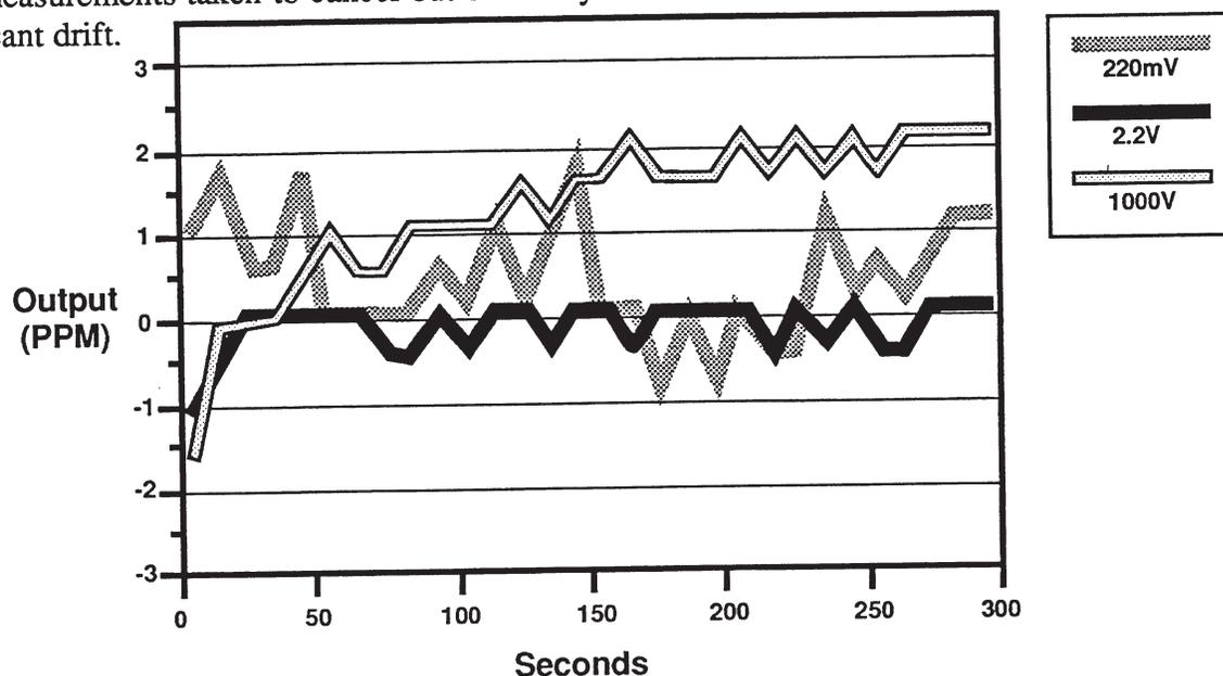
**Figure 4. 792A Output Settling: 220 mV, 2.2 V & 1000 V Ranges**
