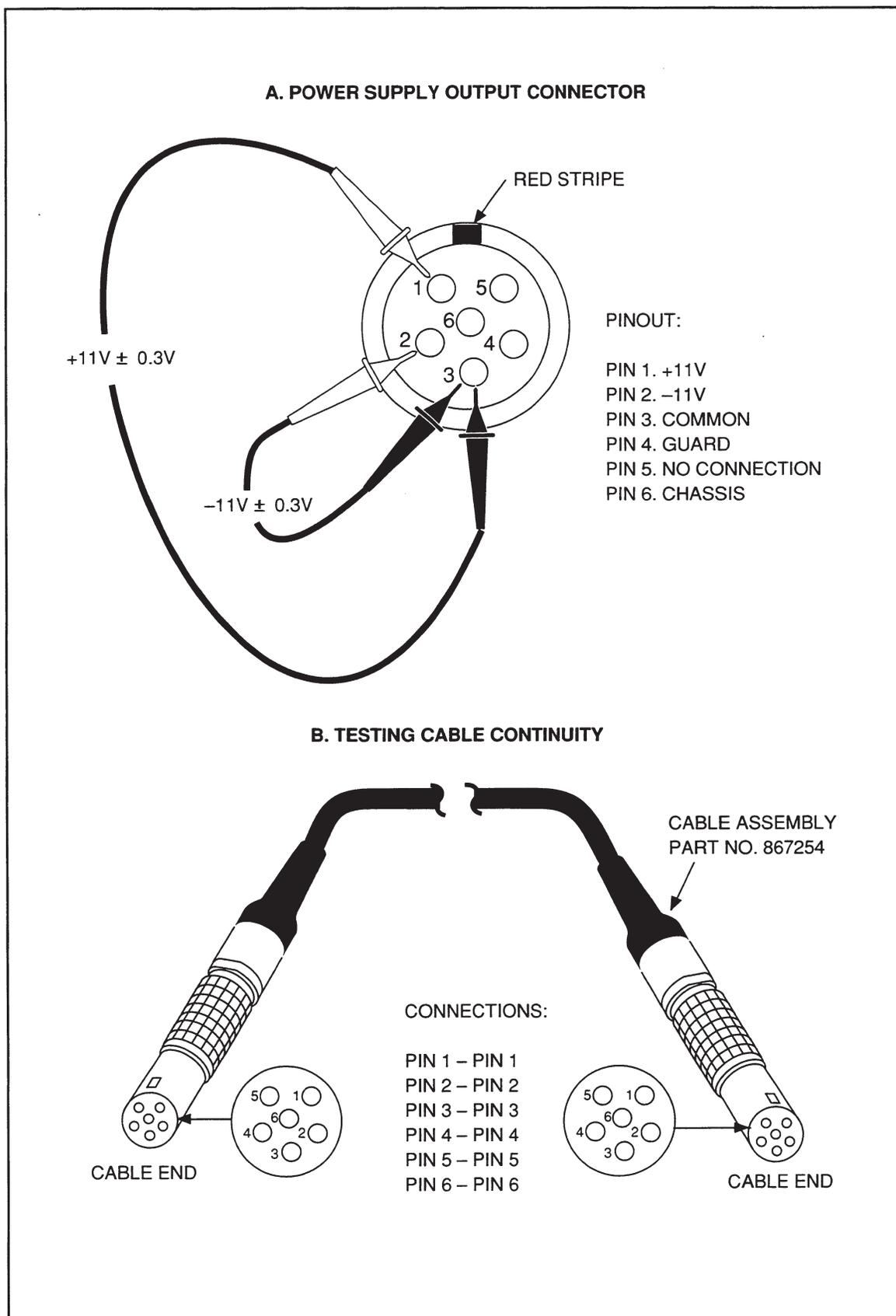
Figure 5-2. Power Pack Cable and Output Voltage
