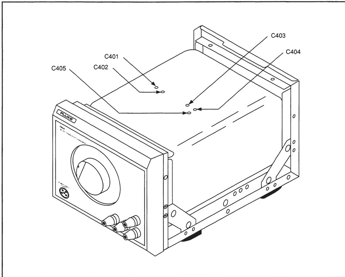
Figure 5-6. Location of Adjustments on the AC Can
