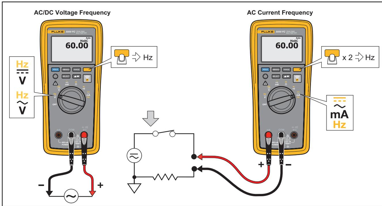
Figure 8. Frequency Measurement
