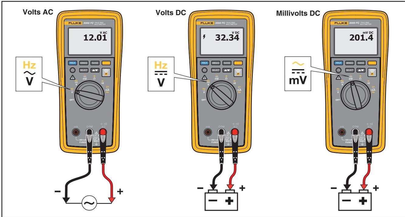
Figure 1. AC and DC Voltage Measurements
