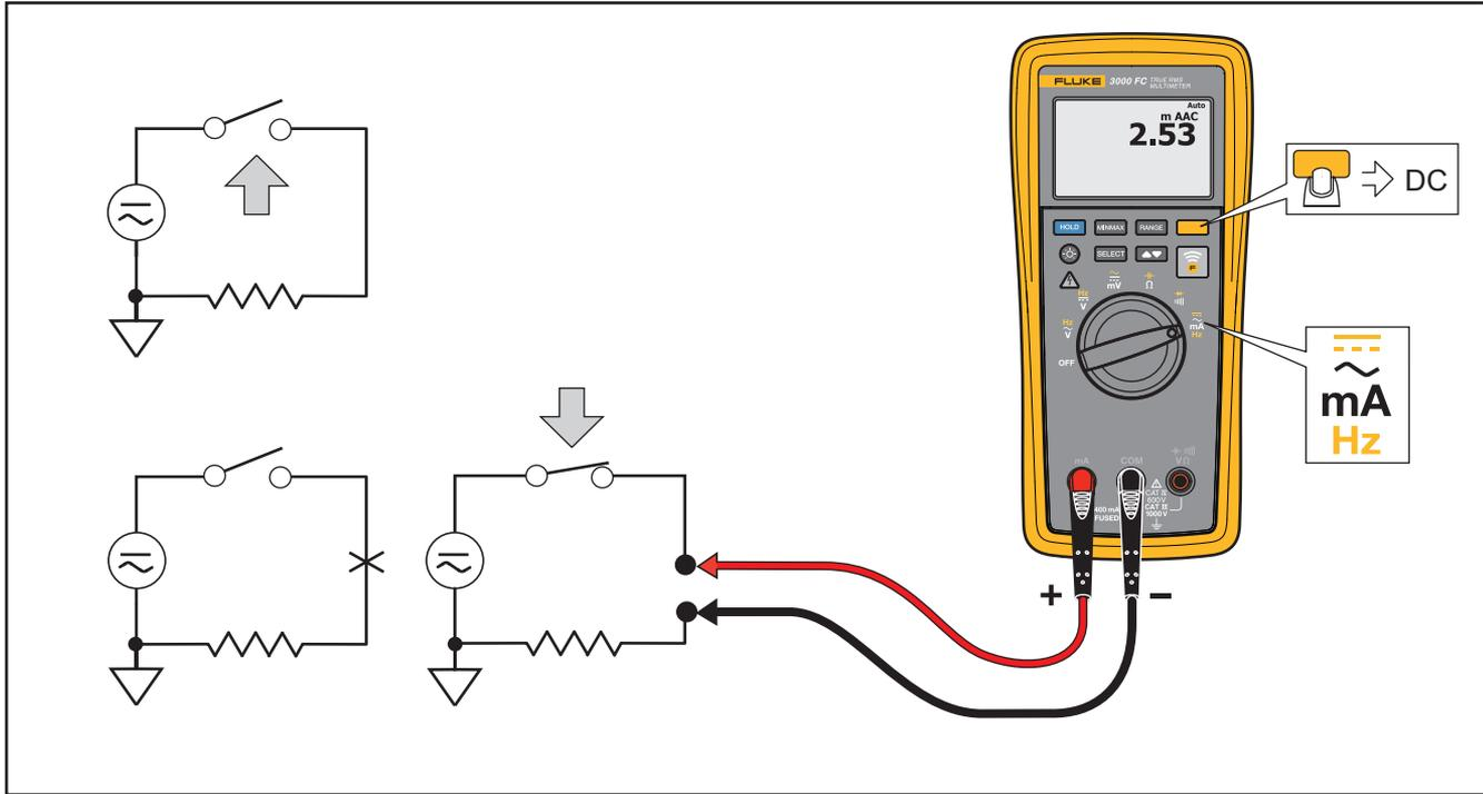
Figure 6. AC and DC Current Measurements
