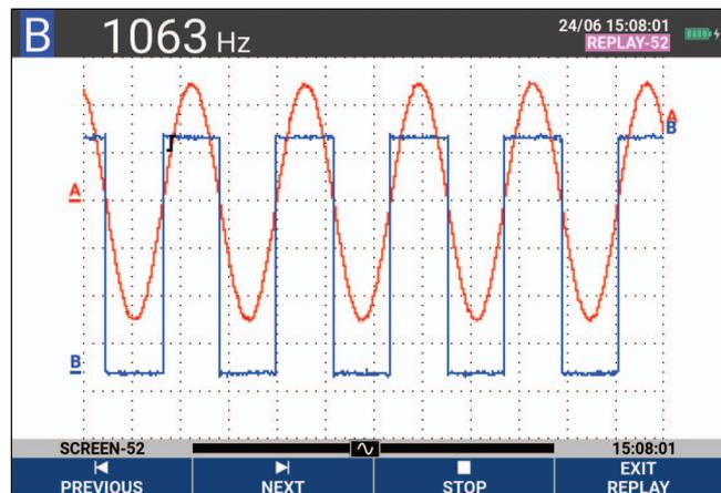
The replay bar represents all 100 stored screens in memory. The icon represents the picture being displayed on the screen (in this example: SCREEN -52). If the bar is partly white, the memory is not completely filled with 100 screens.
