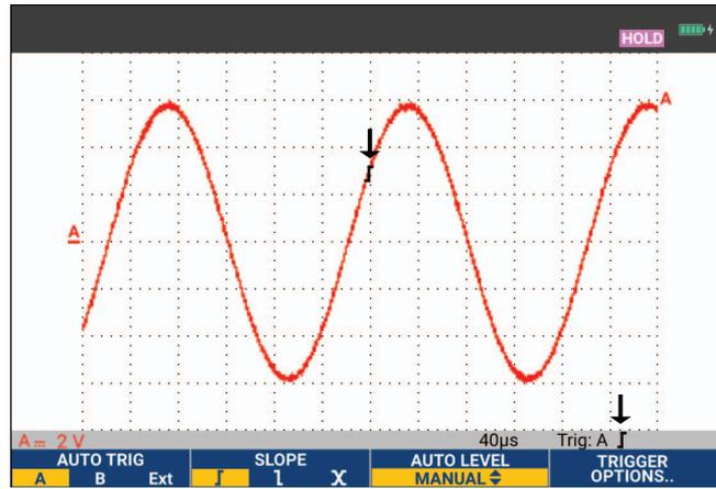
When a valid trigger signal is found, the trigger key will be lit and the trigger parameters appear in black. When no trigger is found, the trigger parameters appear in gray and the key light will be off.
