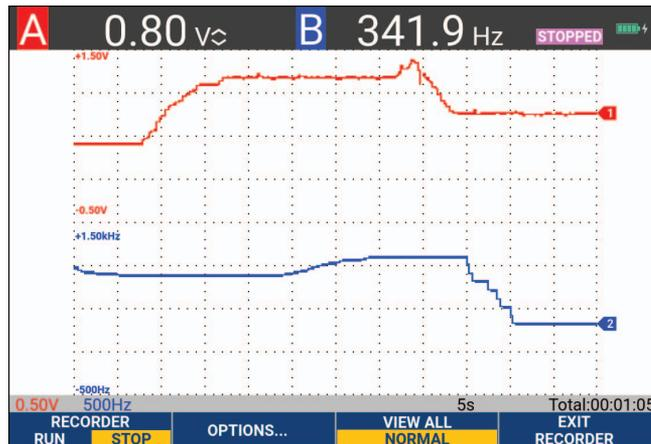
When the test tool is in automatic mode, automatic vertical scaling is used to fit the TrendPlot graph on the screen.
