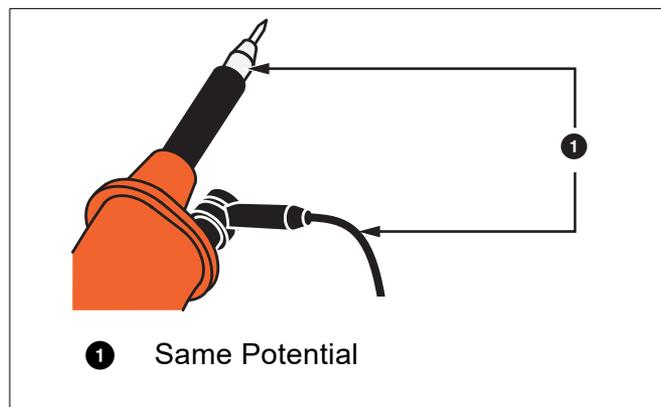
Figure 42. Wrong Connection of Reference Leads
