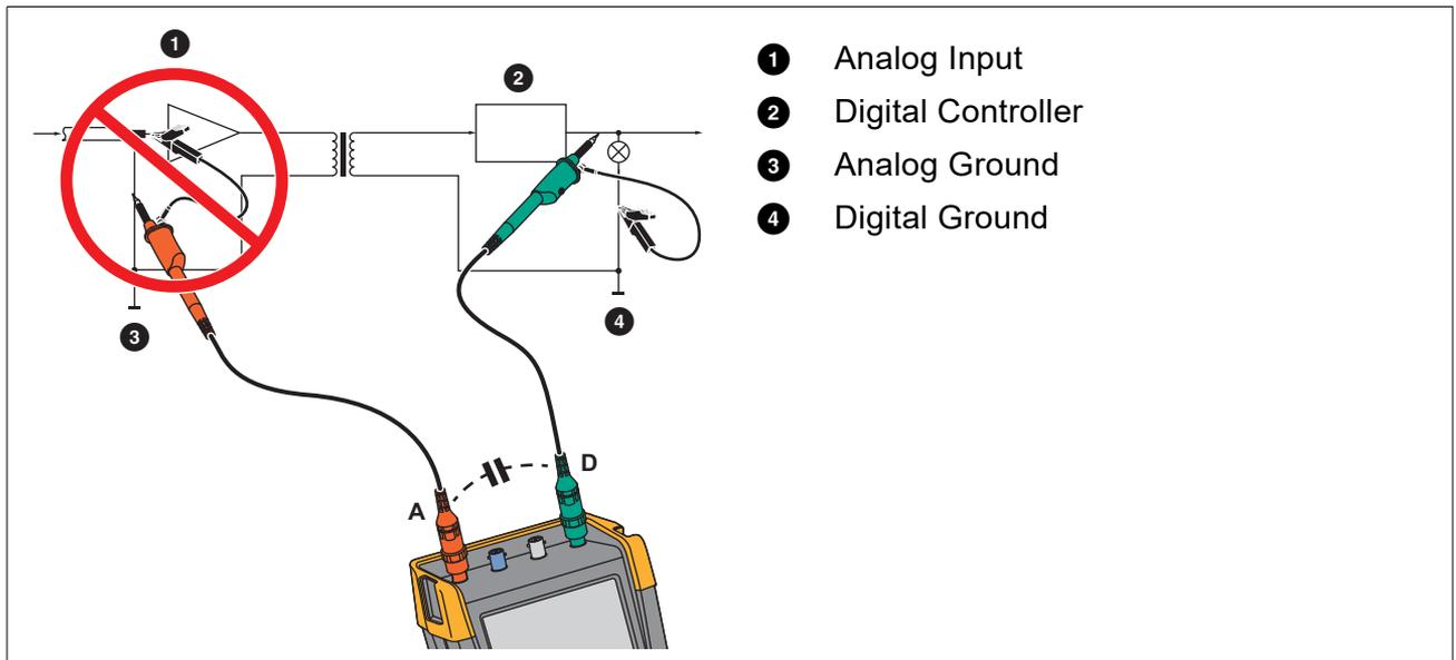
Noise that is picked up by reference lead D can be transmitted by parasitic capacitance to the analog input amplifier.
