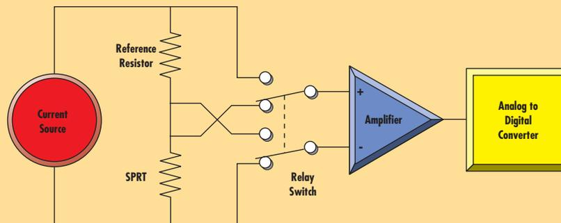
Figure 1. Simplified schematic diagram of the measurement circuit.
