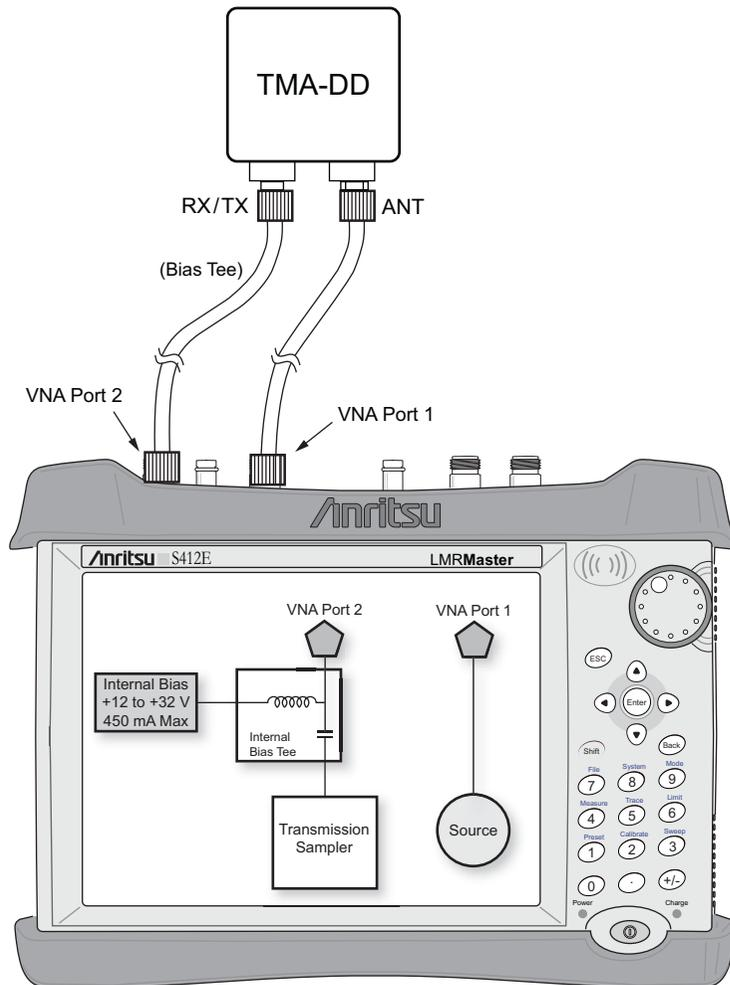
**Figure 8-2.** Bias Tee Setup in VNA Mode
