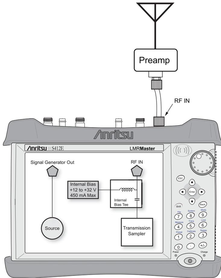
Figure 8-4. Bias Tee Setup in SPA Mode
