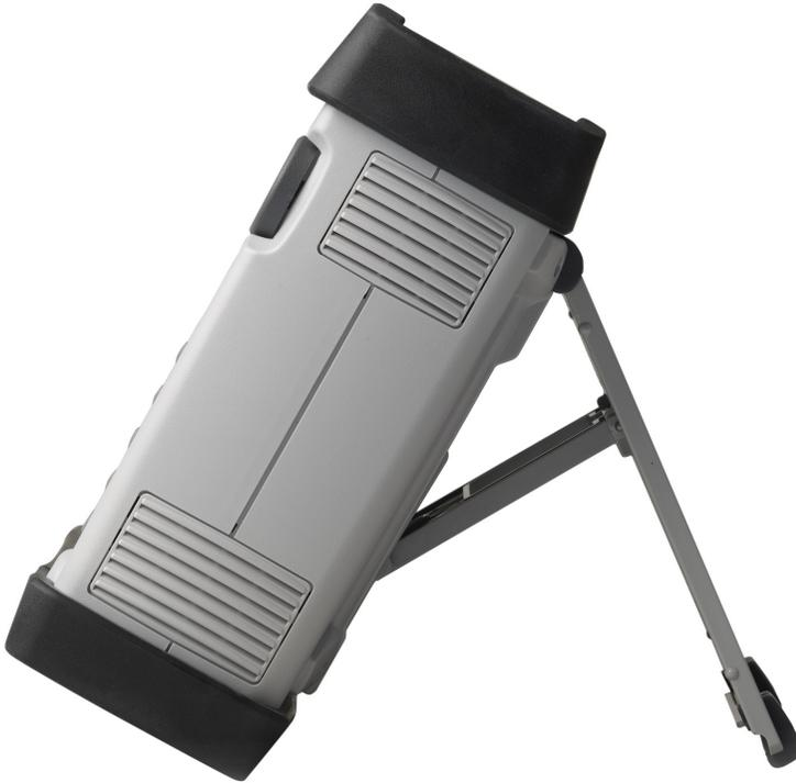
**Figure 2-16.** Tilt Bail—Partly Extended
