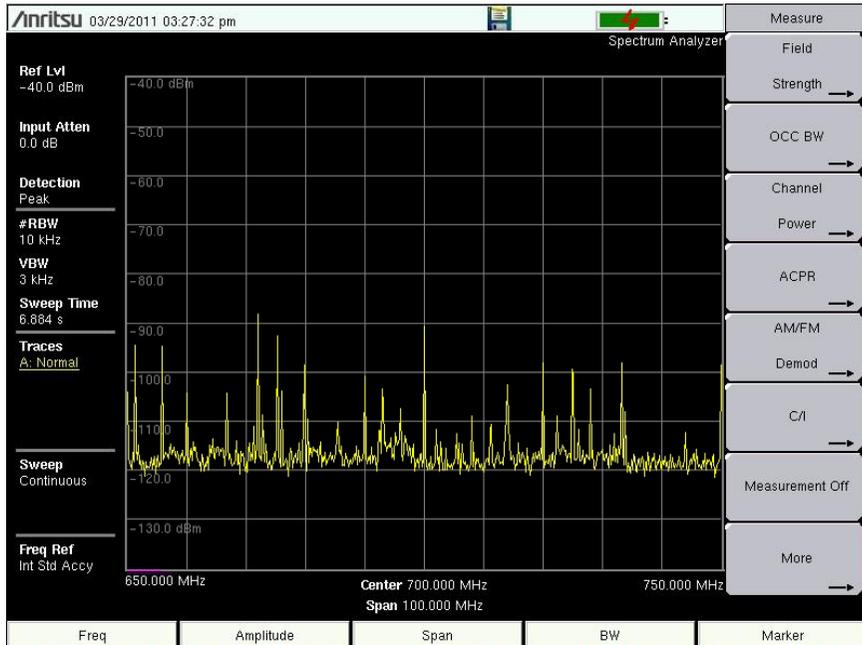
**Figure 3-8.** Spectrum Analyzer Measure Menu with Smart Measurements
