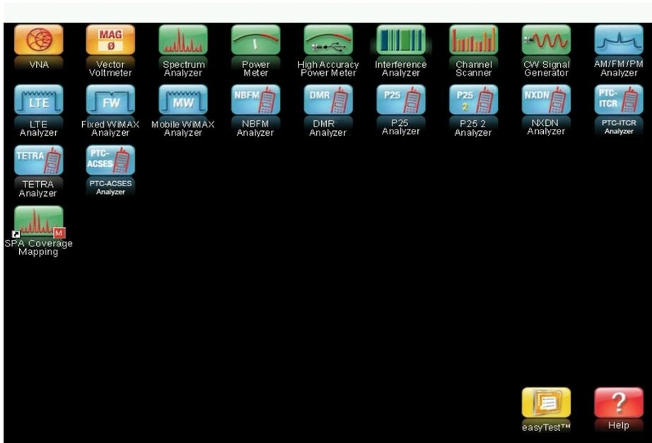
**Figure 2-2.** Menu Key Screen, Icons for Installed Measurements
