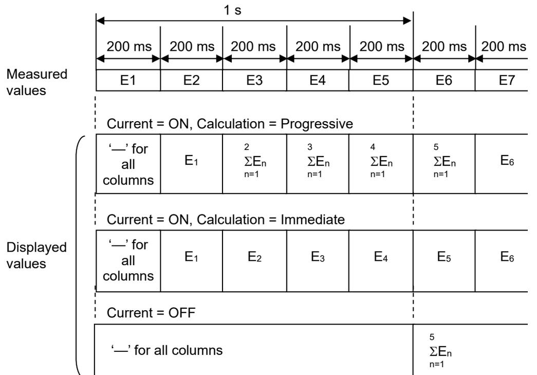
Figure 5.11.2-4 Relationship between measured values and displayed values
