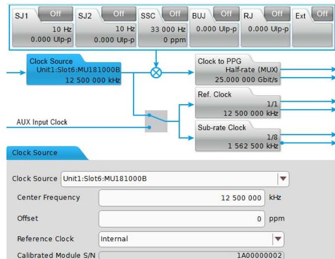
Figure 5.7.1.1-1 MU181500B Clock Source Settings
