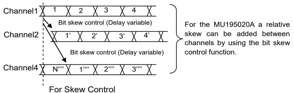
Figure 5.8.2-2 Skew Channel Synchronization Pattern
