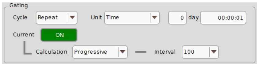
Figure 5.12.1-1 Measurement period setting items in Gating area
