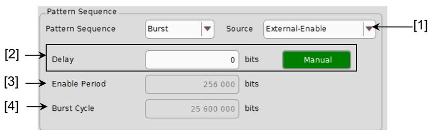
Figure 5.16.1.2-1 Pattern Sequence area when Burst is selected
