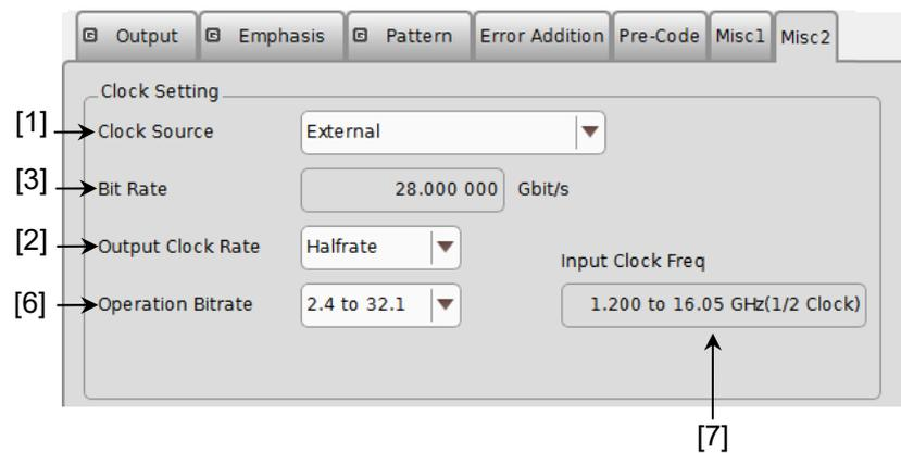
Figure 5.7.1-2 Setting items for Clock setting (when External is selected)
