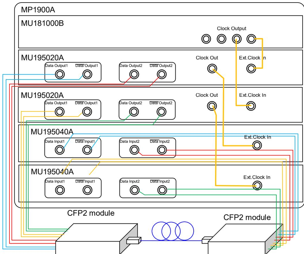
Figure 6.1-1 Connection diagram for CFP2 module evaluation
