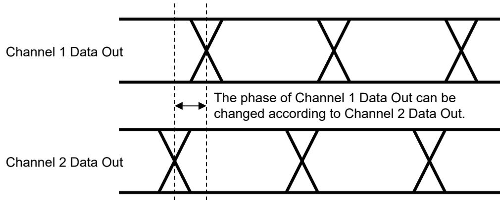
Figure 5.1.2-3 Delay setting in the case of Combination
