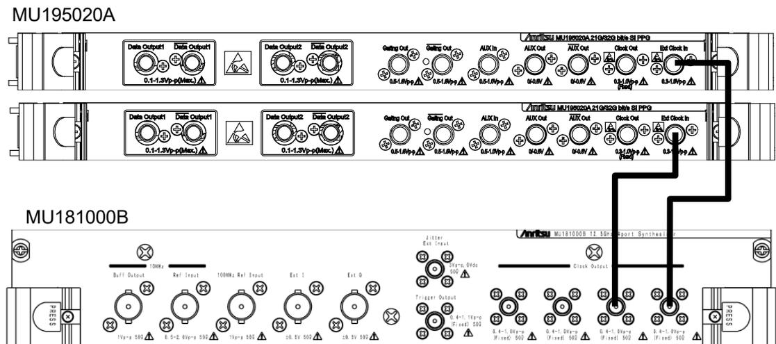
Figure 3.2.4-1 Connection Example for PPG Multi-Channel Synchronization
