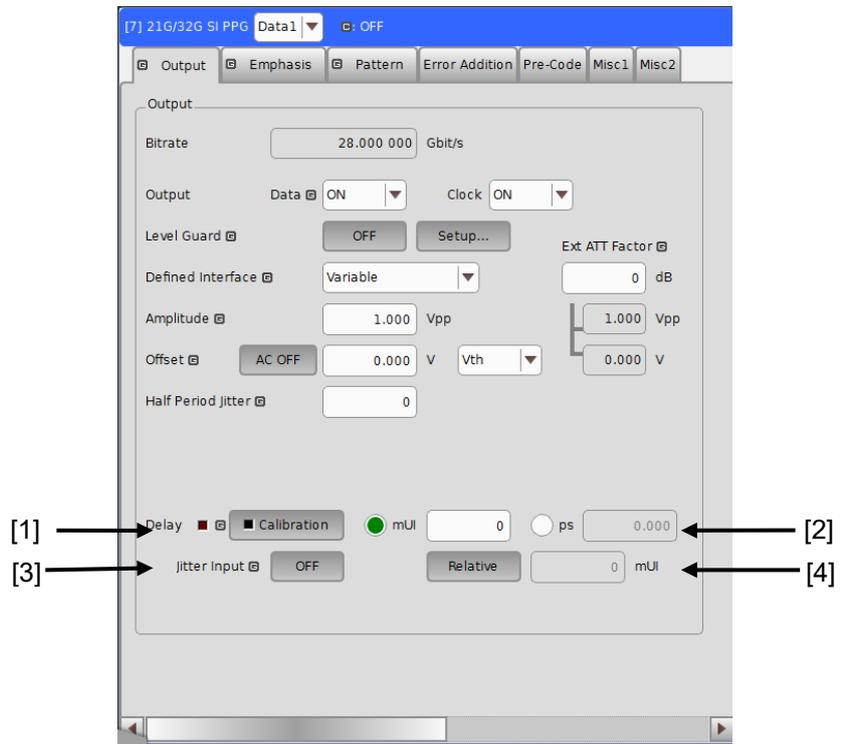
Figure 5.1.2-2 Output Tab When Setting the Delay
