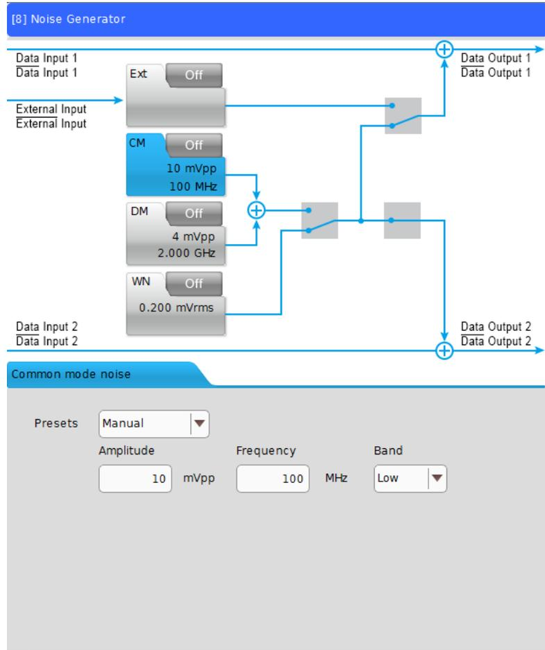
Figure 4.2.3-1 MU195050A function setting
