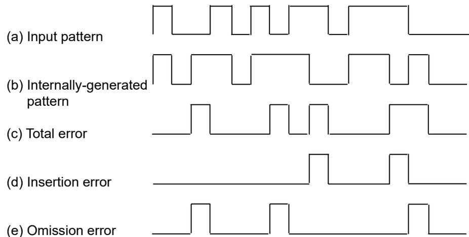
Figure 5.11.3-2 Error detection (Total, Insertion, and Omission errors)
