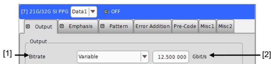
**Figure 5.1.4-1 [Output] Tab Bit Rate Setting Area**
