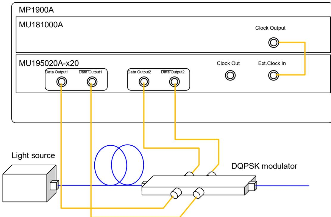
Figure 6.2-1 Connection diagram for generating 56 Gbit/s DQPSK signals
