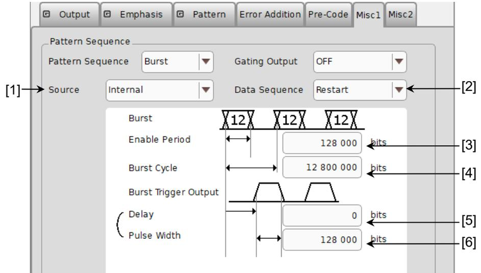
Figure 5.6.1.2-1 Setting items for Burst pattern sequence
