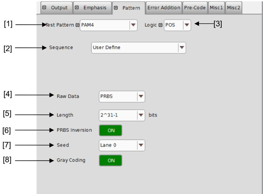
Figure 5.3.6-2 Setting Items for Test Pattern (PAM4-PRBS)
