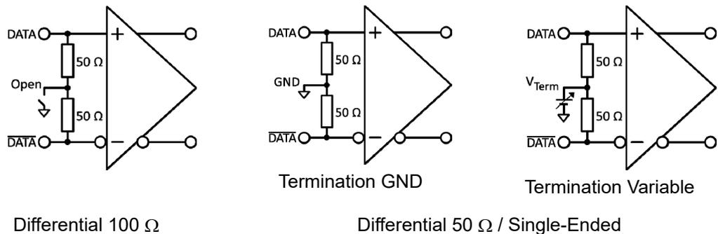
Figure 5.14.1-3 Termination Methods in Different Setups
