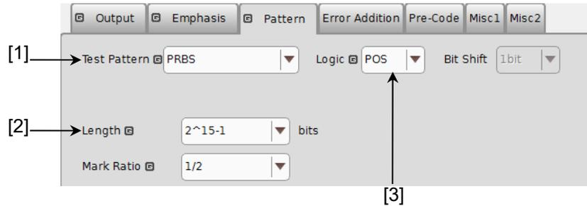
Figure 5.3.2-1 Setting items for Test Pattern (PRBS)
