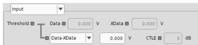
Figure 5.11.1-2 Input voltage threshold difference setting items
