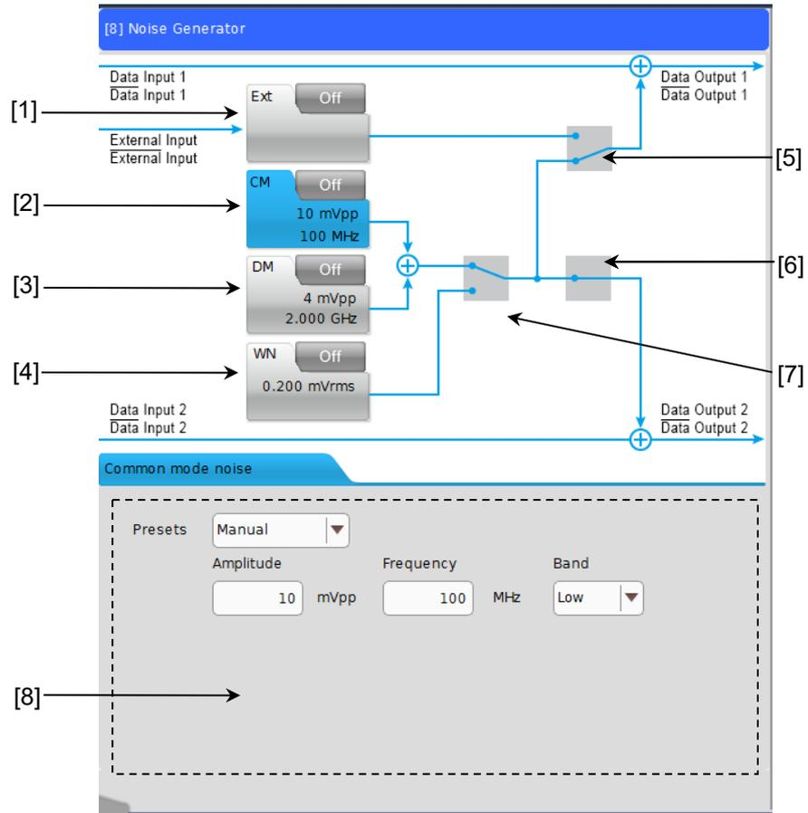
Figure 5.20.1-1 MU195050A Operation Window
