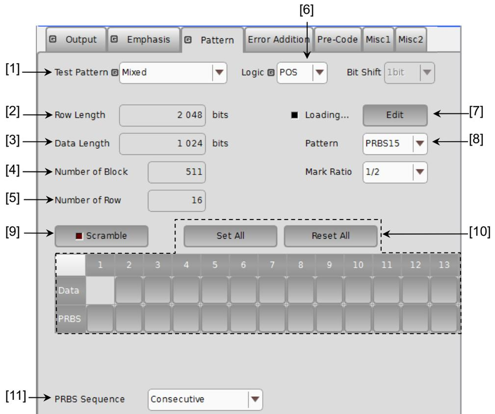
**Figure 5.3.5-1 Setting items for Test Pattern (Mixed Data)**
