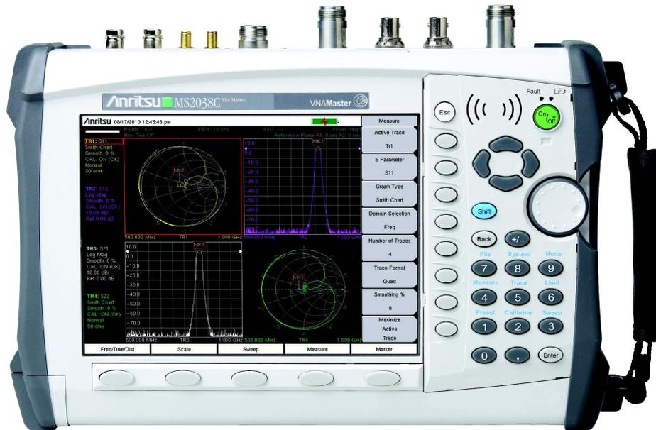
VNA Master™ MS202xC/MS203xC Vector Network Analyzer + Spectrum Analyzer
