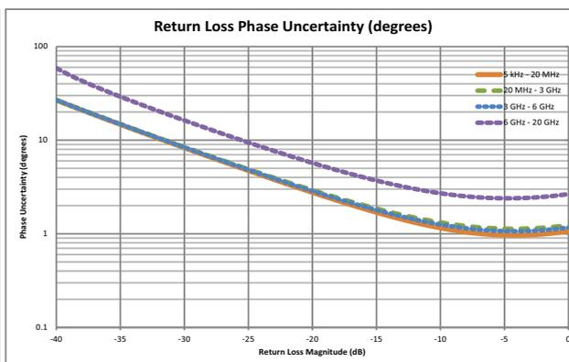
1. Full 2-Port calibration, Default Power, 10 Hz IFBW, No averaging, 10 minute warm-up. TOSLKF50A-20 or TOSLKF50A-40 calibration kit. Load match specification applicable directly at corrected port only. De-rate by approximately 8 dB if using a 3670 series test port cable. Reflection and Transmission Tracking are typical.
