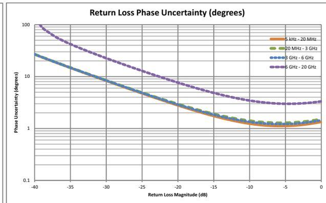
1. Full 2-Port calibration, Default Power, 10 Hz IFBW, No averaging, 10 minute warm-up. OSLN50A-18 or TOSLN50A-18 calibration kit. Load match specification applicable directly at corrected port only. De-rate by approximately 8 dB if using a 3670 series test port cable. Reflection and Transmission Tracking are typical.
