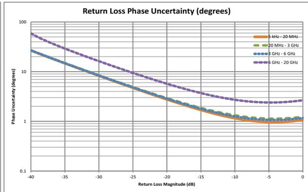
1. Full 2-Port calibration, Default Power, 10 Hz IFBW, No averaging, 10 minute warm-up. TOSLK50A-20 or TOSLK50A-40 calibration kit. Load match specification applicable directly at corrected port only. De-rate by approximately 8 dB if using a 3670 series test port cable. Reflection and Transmission Tracking are typical.
