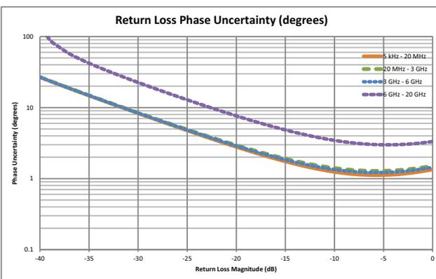
1. Full 2-Port calibration, Default Power, 10 Hz IFBW, No averaging, 10 minute warm-up. OSLNF50A-18 or TOSLNF50A-18 calibration kit. Load match specification applicable directly at corrected port only. De-rate by approximately 8 dB if using a 3670 series test port cable. Reflection and Transmission Tracking are typical.
